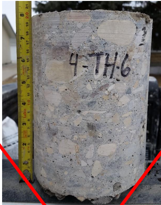
TH06 – 200 mm intact, 30 mm asphalt layer not shown
