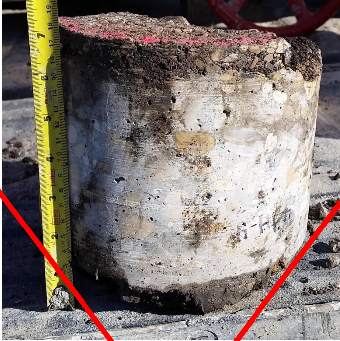
TH04 – 150 mm intact, 30 mm asphalt layer
