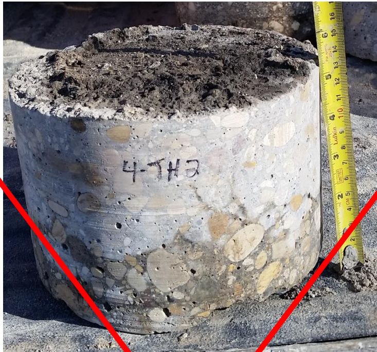
TH02 – 140 mm intact, 40 mm asphalt layer not shown
