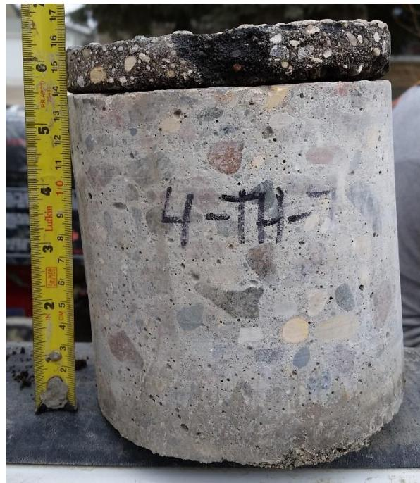
**TH07** – 140 mm intact, 20 mm asphalt layer
