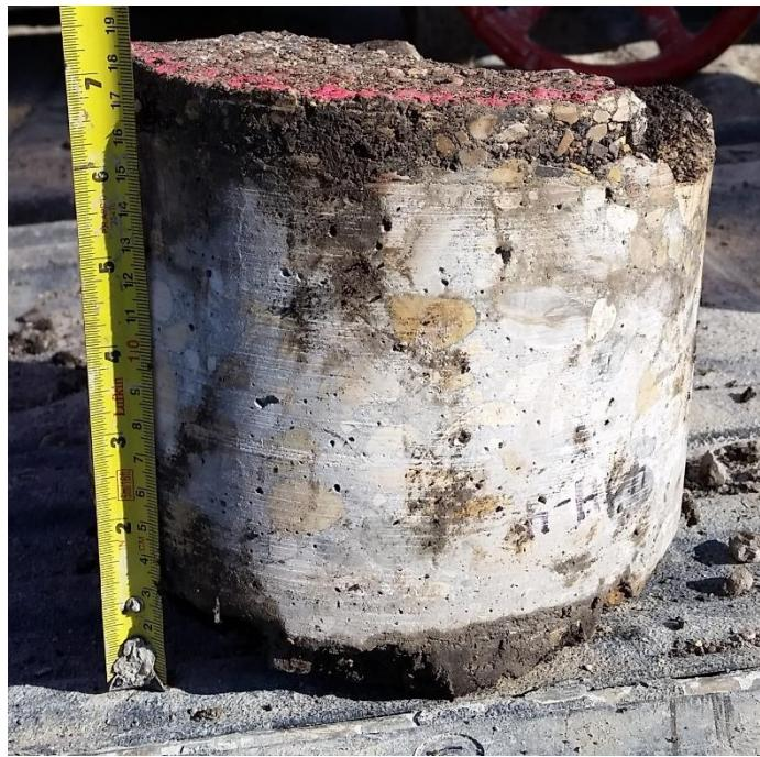
**TH04** – 150 mm intact, 30 mm asphalt layer
