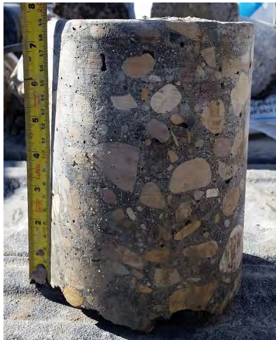
Figure 36: TH35 – 190 mm intact concrete
