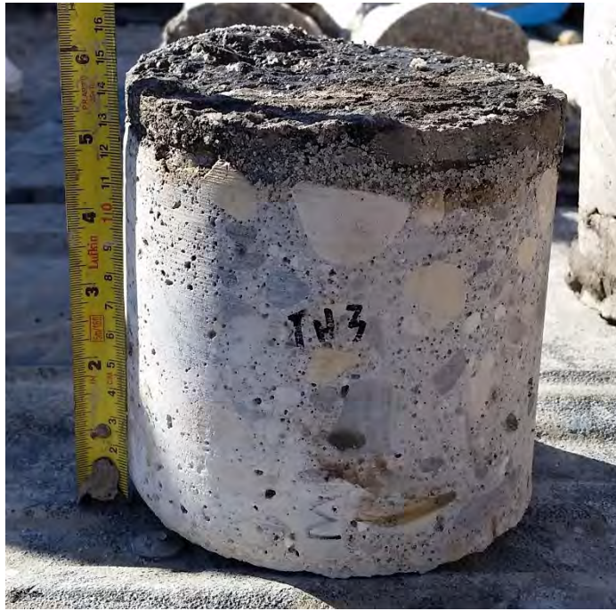
Figure 31: TH31 – 20 mm asphalt, 130 mm intact concrete
