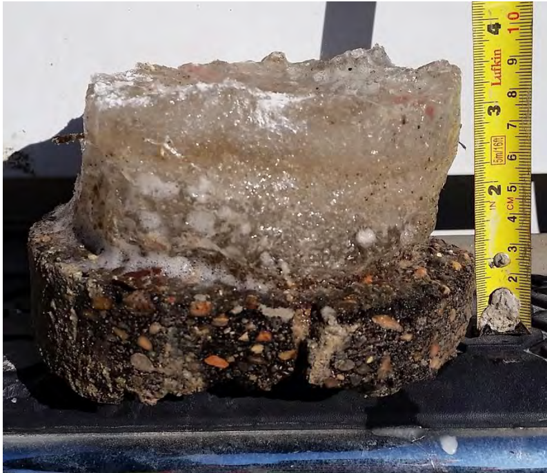
Figure 3: TH3 – 30 mm asphalt, no concrete
