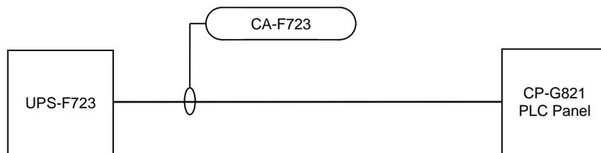
**Figure 7-2: Instrument Cable Identification Example – Identified Equipment**
