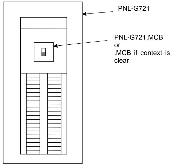
**Figure 2-3 : Electrical Subcomponent Example – Main Circuit Breaker**
