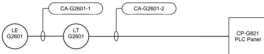
**Figure 7-1: Instrument Cable Identification Example – Level Transmitter**
