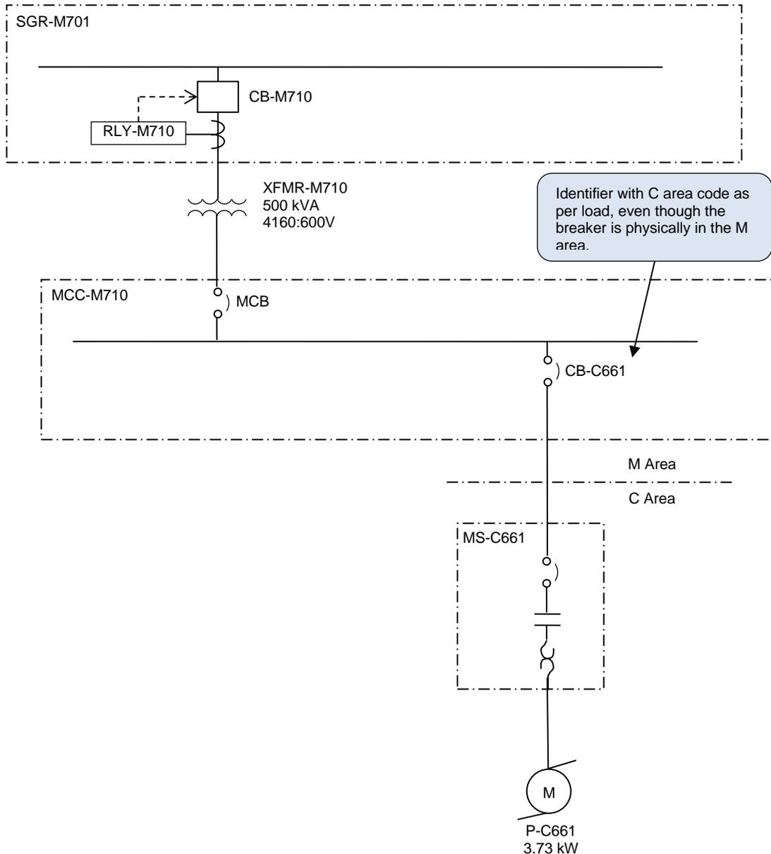
**Figure 6-3 : Example Identification by Load Equipment**
