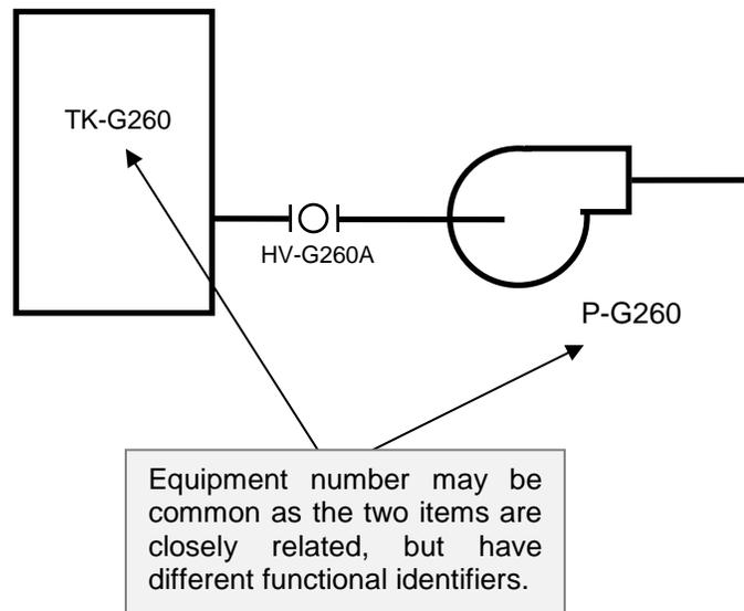
**Figure 2-1: Equipment Number Example – Functionally Related**
