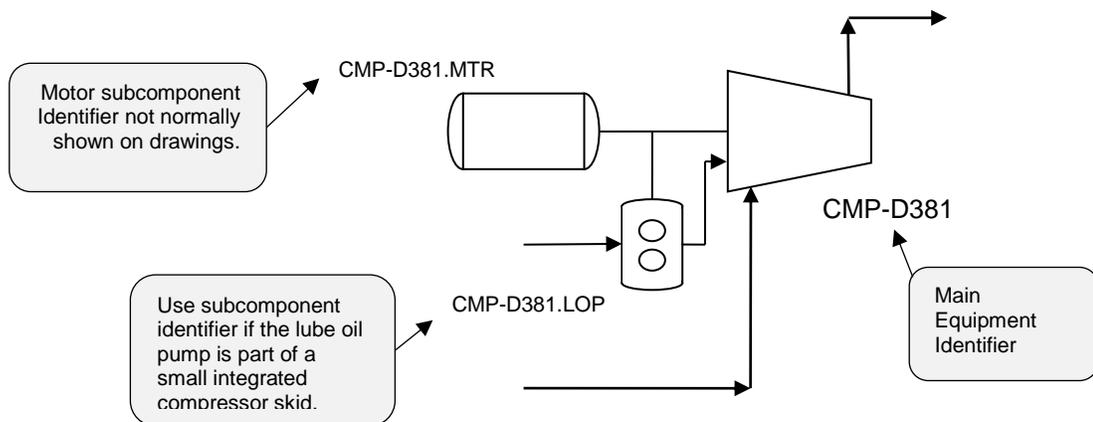
**Figure 2-2 : Lube-Oil Pump Subcomponent Example**
