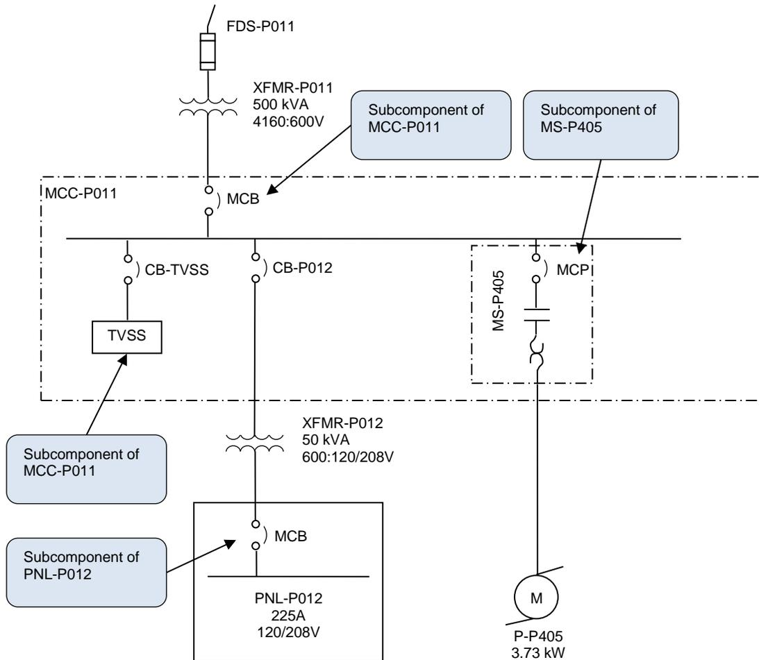
**Figure 6-2 : Subcomponents – Electrical Equipment**
