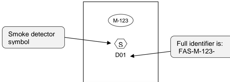
**Figure 6-4 : Room Numbering on Drawings – Plan View**
