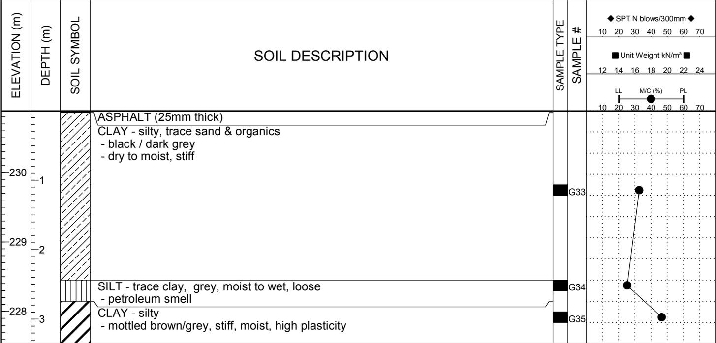
END OF TEST HOLE AT 3.4 m IN CLAY
