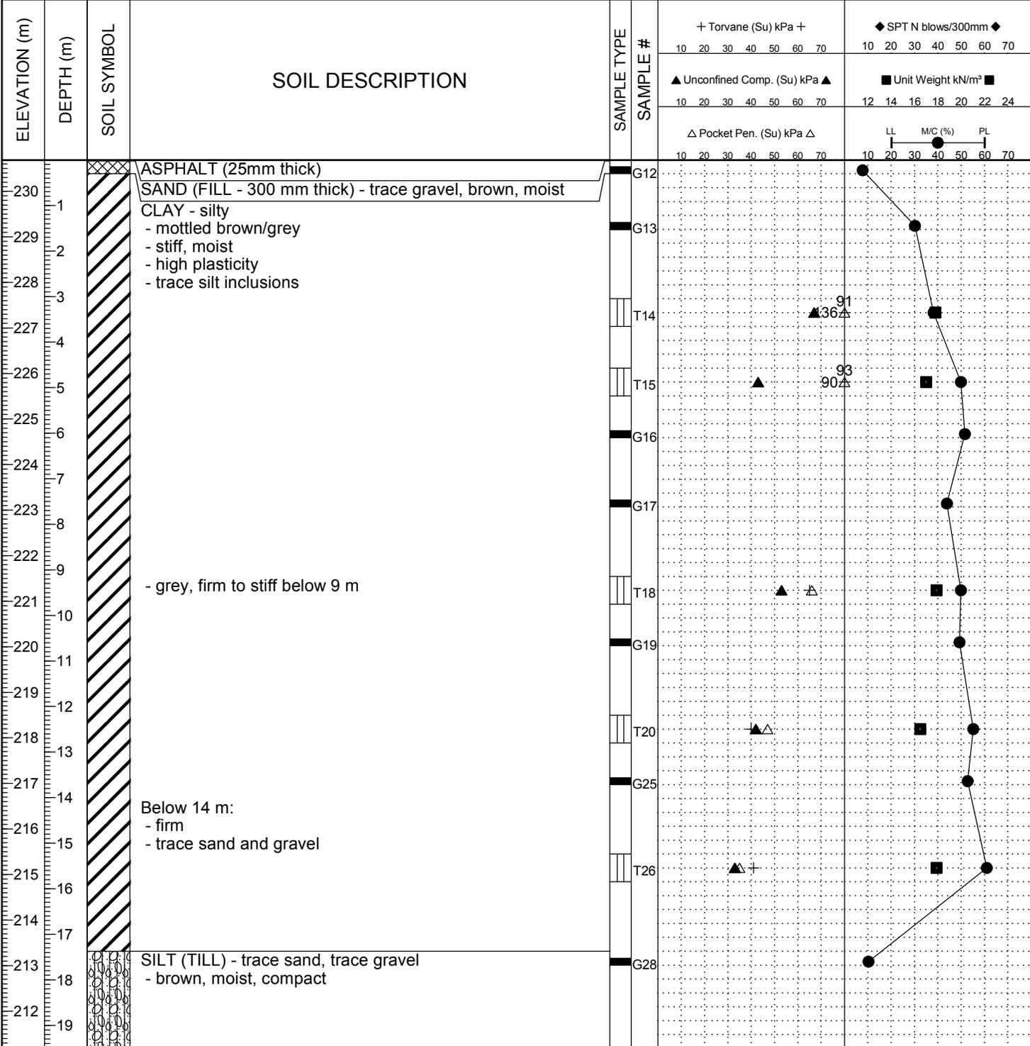
END OF TEST HOLE AT 19.5 m IN SILT (TILL) (AUGER REFUSAL)
