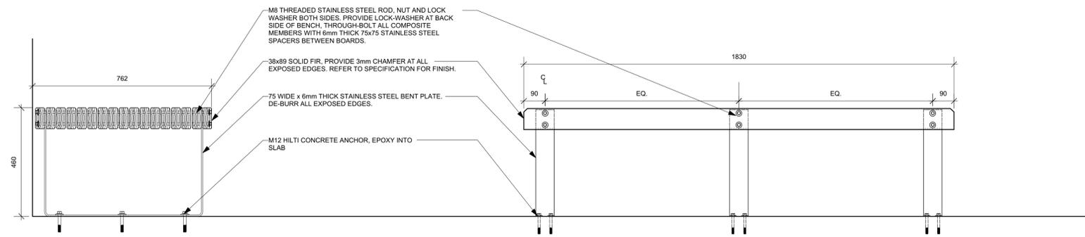
NOTE: CONTRACTOR TO SCAN FLOOR PRIOR TO FABRICATION. ADJUST ANCHOR LOCATION TO NOT CONFLICT WITH REBAR
