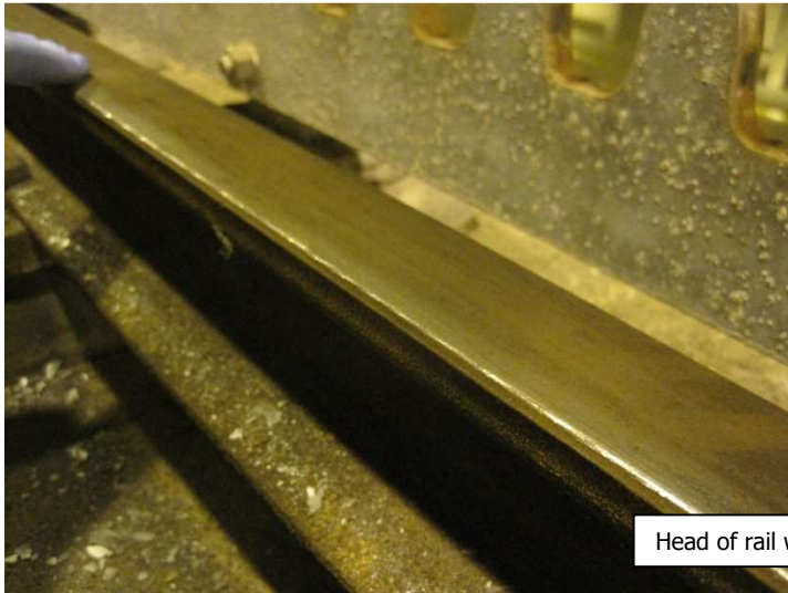
Overlay from flattened rail head has begun to delaminate in certain sections
