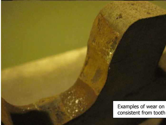
Examples of damaged cog track teeth
