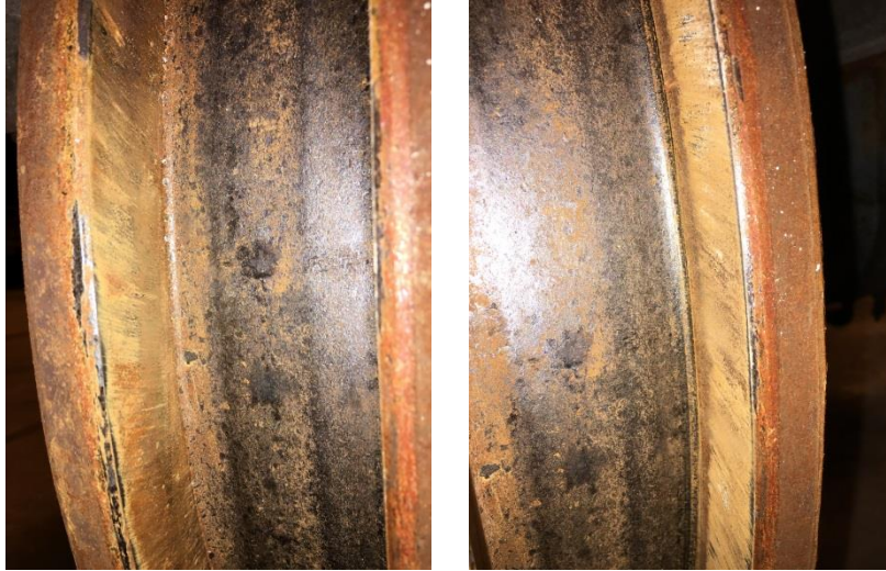
Figure 6: Wear on North End-Truck Wheels
