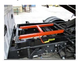
All components (prop, handle and receiving bracket) shall be painted with **Safety Orange** for ease of identification
