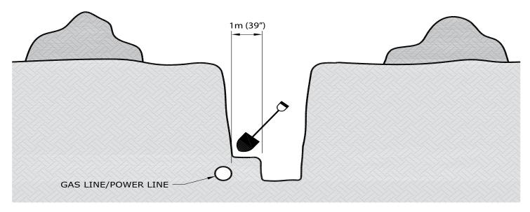
Dig a trench or bell hole 1 metre (39 inches) from the line location, parallel to the line, then hand dig laterally to expose the line.
