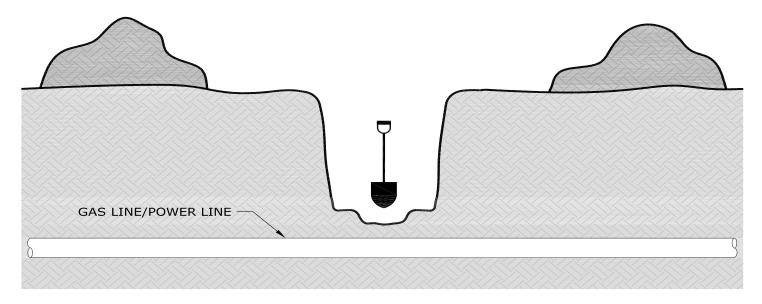
Dig a trench by hand across the full width of the excavation (perpendicular to or "across from" the line). If the line is not uncovered, mechanically excavate to one half the depth of the trench. Repeat this process until the line is exposed.
