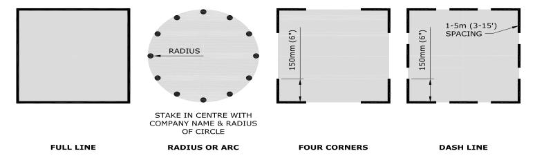
If an excavation is contained within a 5 metre (16 feet) maximum radius then it can be marked with a single white stake at the centre of the excavation. The stake must clearly state the company identifier and the radius of the excavation in black lettering. This information must be conveyed to Manitoba Hydro.
