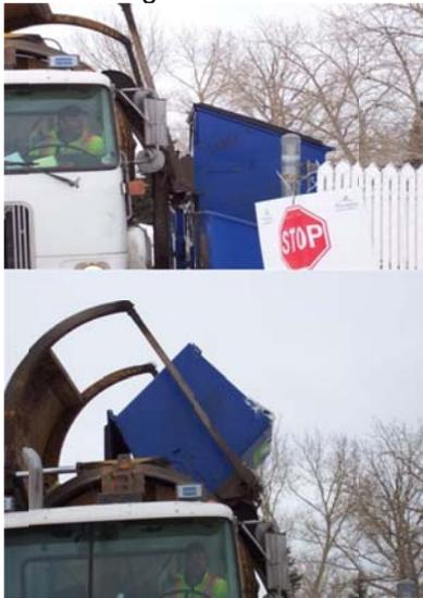
The City of Winnipeg currently utilizes the side-load container system for its recycling operation. The containers have been modified for maximum on-site storage capacity; they are serviced in reverse of their original design. As shown in the attached photos, the high side of the container is the front of the container and is the first side to enter into the truck body. See photos for visual reference.
