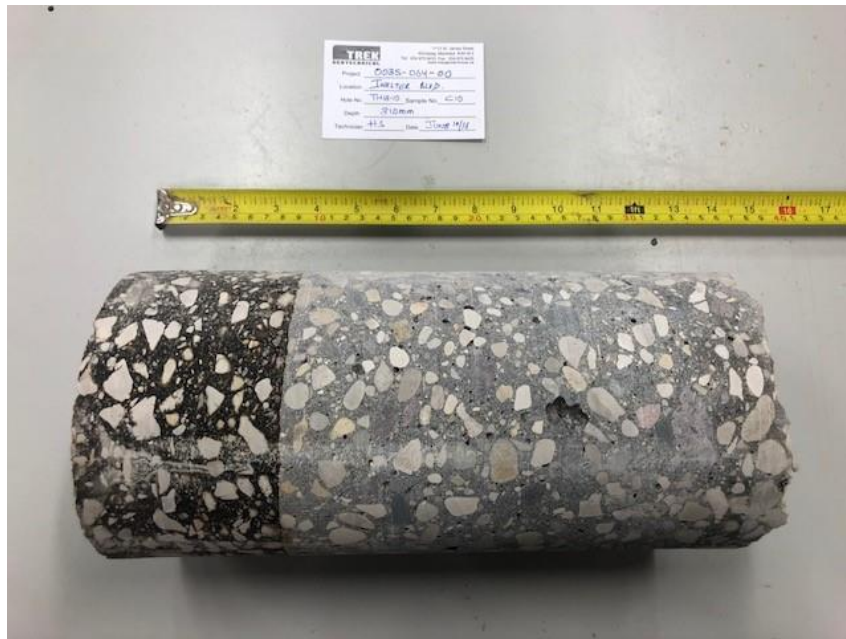
Photo 10: Pavement Core Sample at Test Hole TH18-10
