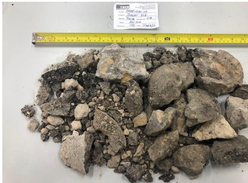
Photo 2: Pavement Core Sample at Test Hole TH18-02
