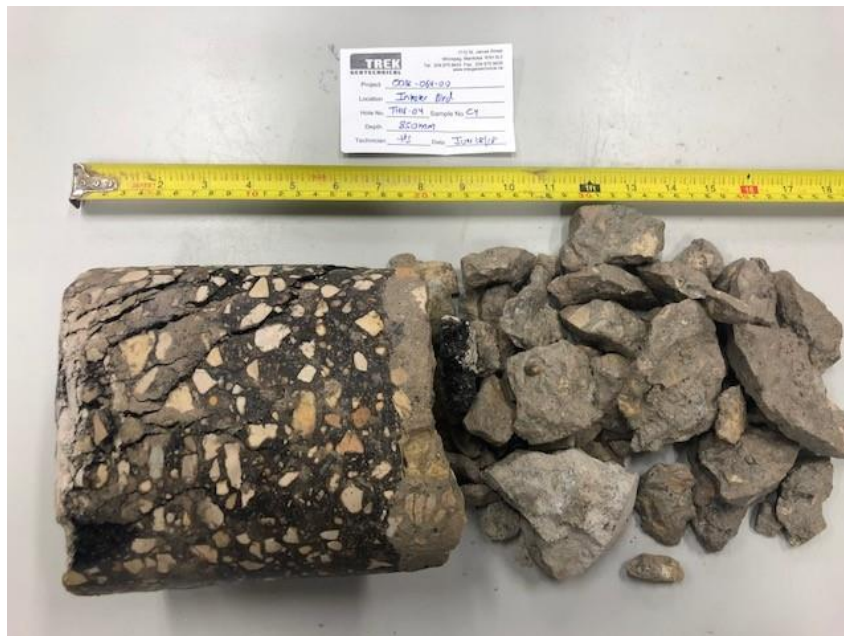
Photo 4: Pavement Core Sample at Test Hole TH18-04
