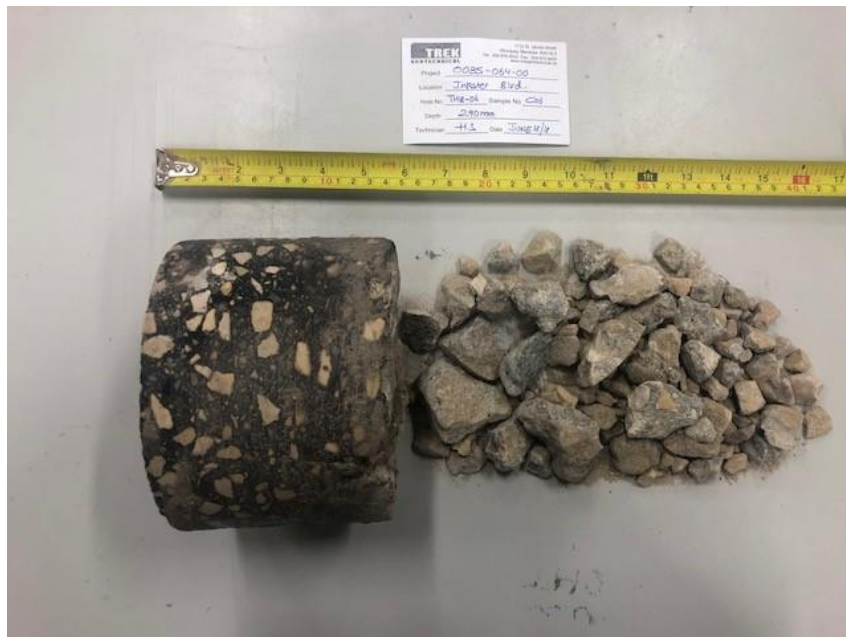
Photo 6: Pavement Core Sample at Test Hole TH18-06
