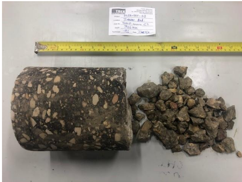
Photo 7: Pavement Core Sample at Test Hole TH18-07
