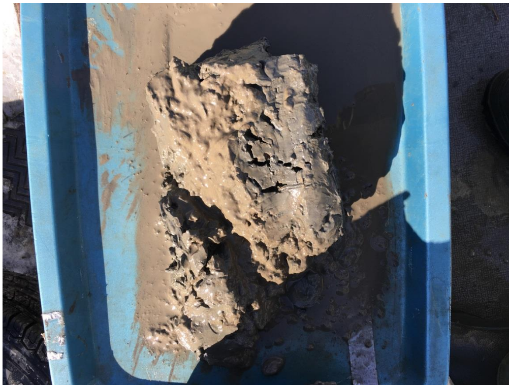
Photo 14. Substrate validation at site T15-20m showing a mix of soft clay/silt.
