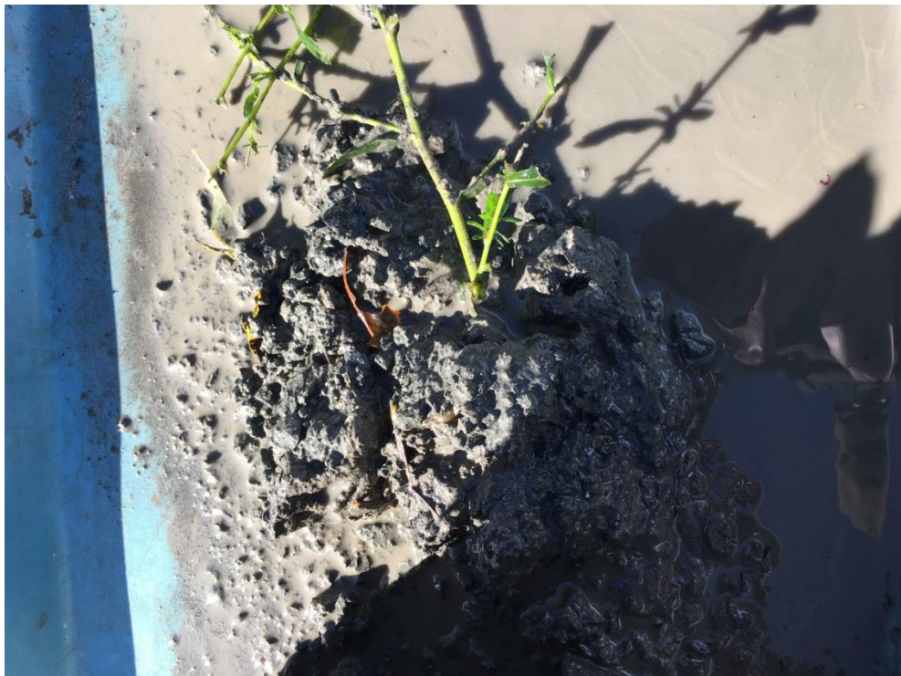
Photo 10. Substrate validation from site T9-15m showing a mix of soft clay/silt and organic material.
