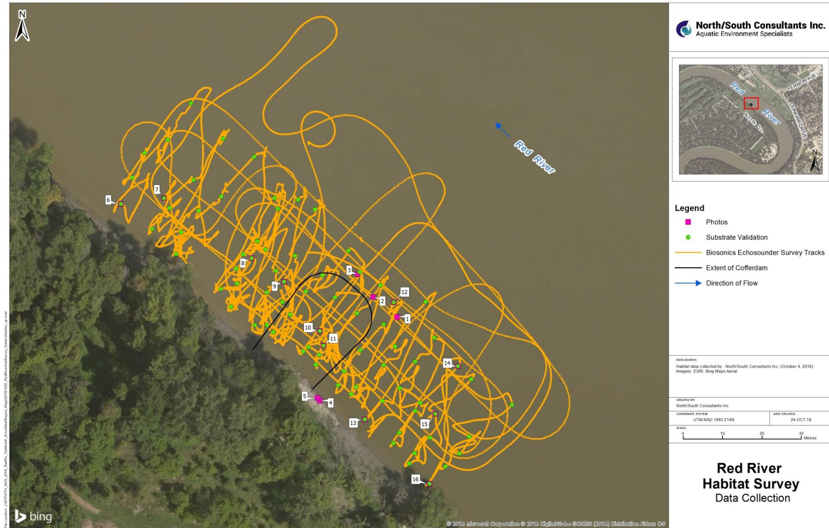
Figure 4. Substrate validation results showing ponar locations and GPS tracks at the Red River North Drive outfall study site.
