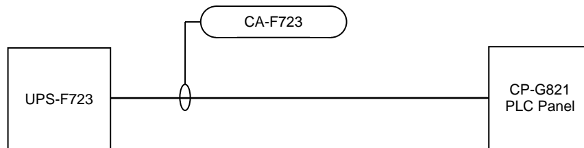
Figure 7-3: Instrument Cable Identification Example – Identified Equipment
