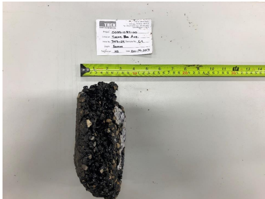
Photo 4: Pavement Core Sample at Test Hole TH17-04
