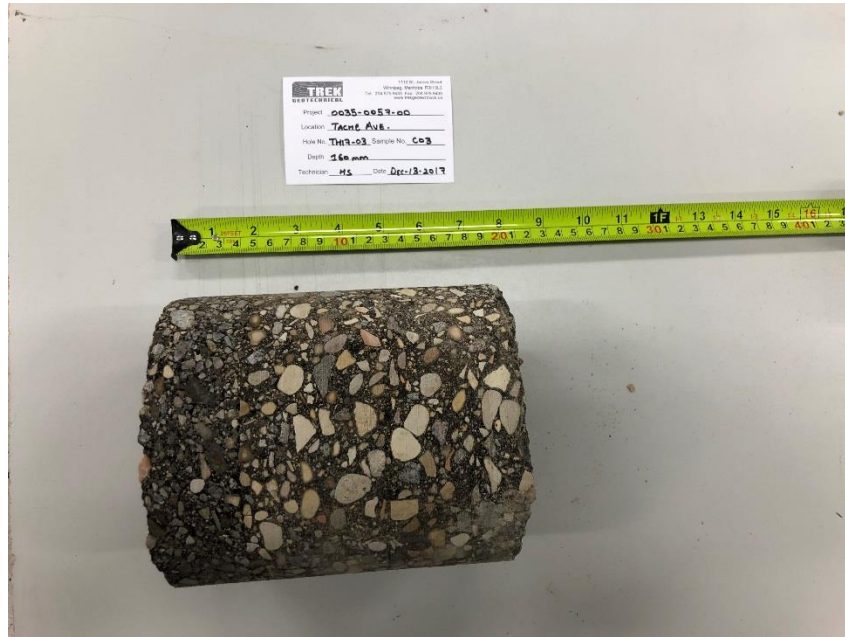
Photo 3: Pavement Core Sample at Test Hole TH17-03
