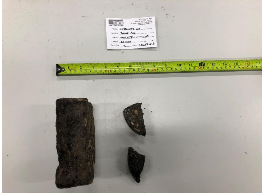
Photo 7: Pavement Core Sample at Test Hole TH17-07
