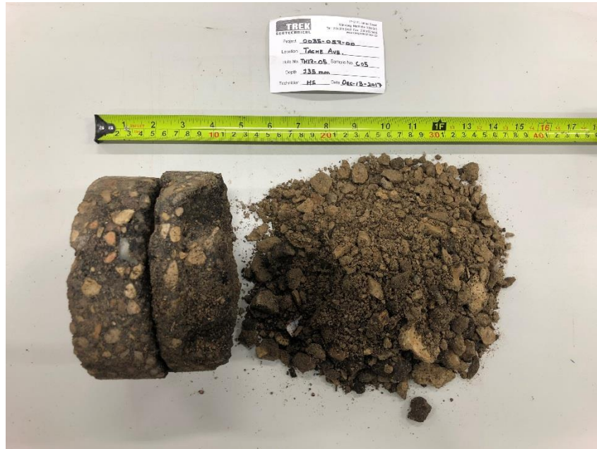
Photo 5: Pavement Core Sample at Test Hole TH17-05
