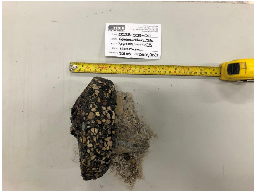
Photo 5: Pavement Core Sample at Test Hole TH17-05
