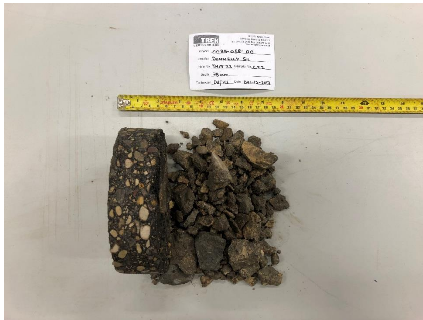
Photo 6: Pavement Core Sample at Test Hole TH17-22
