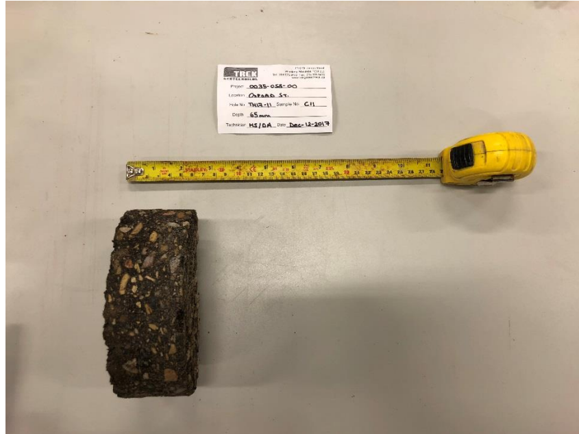
Photo 3: Pavement Core Sample at Test Hole TH17-11
