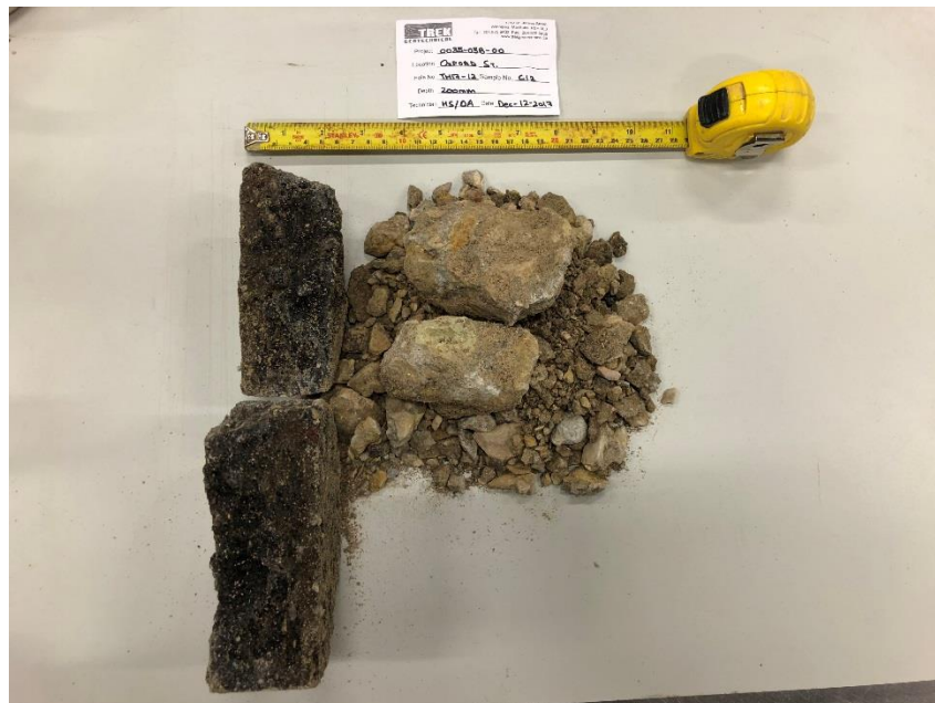
Photo 4: Pavement Core Sample at Test Hole TH17-12
