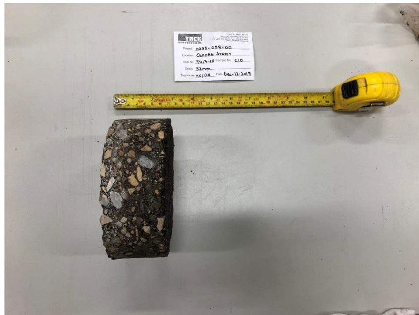
Photo 2: Pavement Core Sample at Test Hole TH17-10
