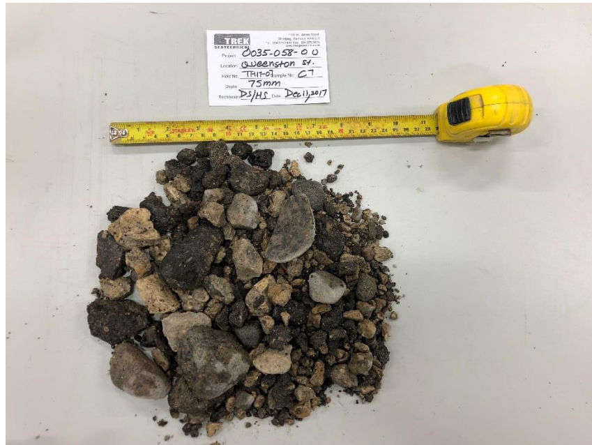
Photo 7: Pavement Core Sample at Test Hole TH17-07
