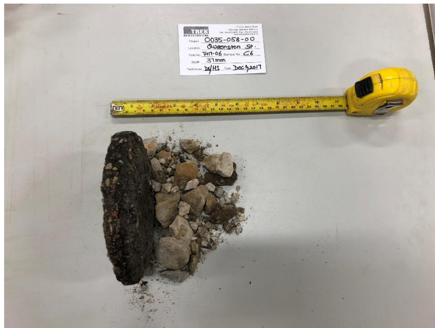
Photo 6: Pavement Core Sample at Test Hole TH17-06
