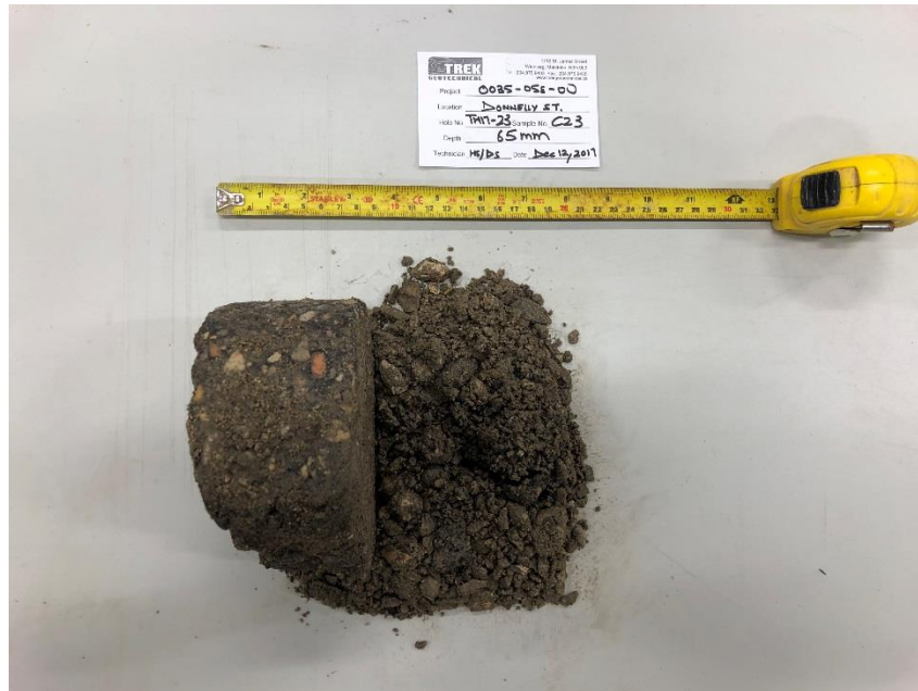
Photo 7: Pavement Core Sample at Test Hole TH17-23
