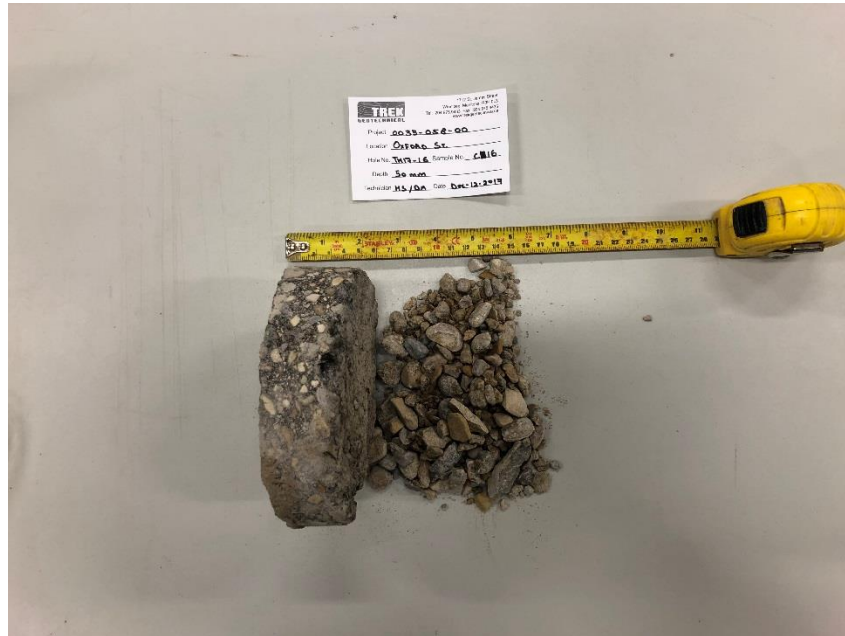
Photo 7: Pavement Core Sample at Test Hole TH17-16
