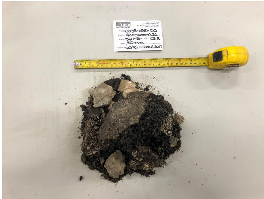
Photo 3: Pavement Core Sample at Test Hole TH17-03
