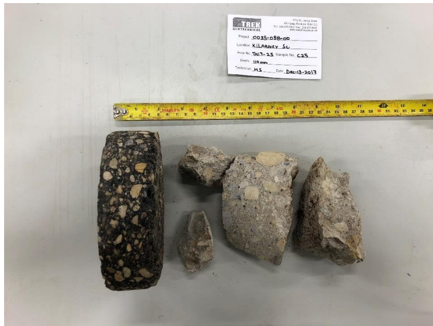
Photo 2: Pavement Core Sample at Test Hole TH17-25
