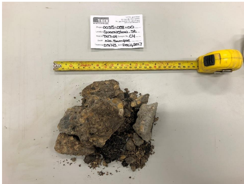
Photo 4: Pavement Core Sample at Test Hole TH17-04
