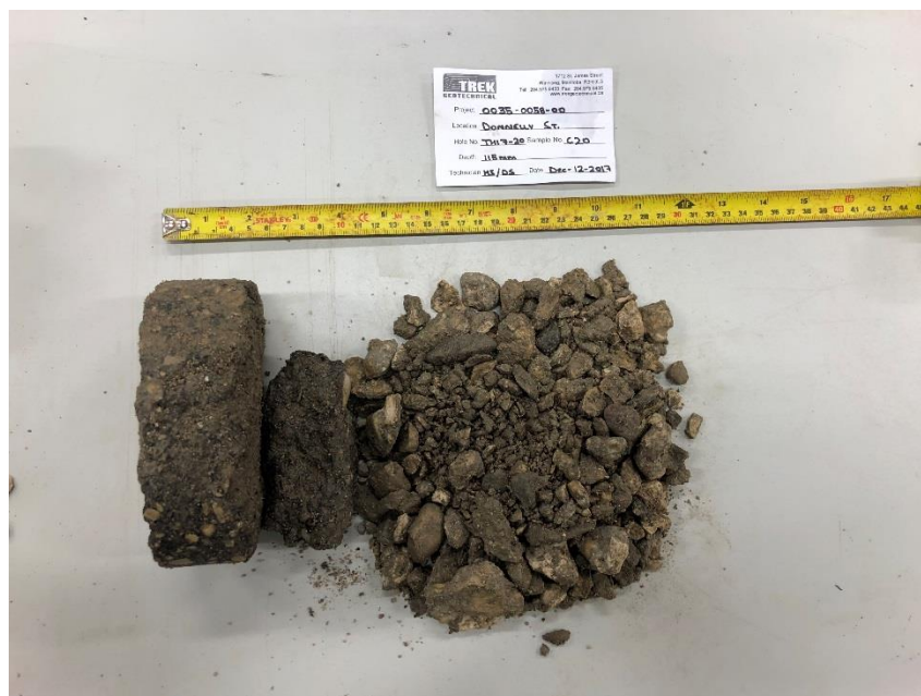
Photo 4: Pavement Core Sample at Test Hole TH17-20
