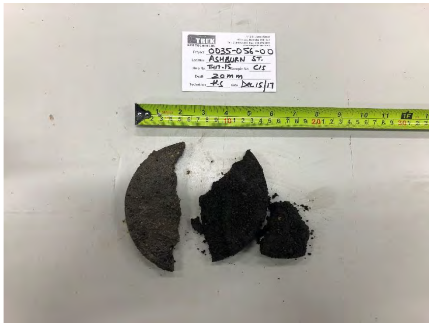
Photo 6: Pavement Core Sample at Test Hole TH17-15 (no recovery of concrete)
