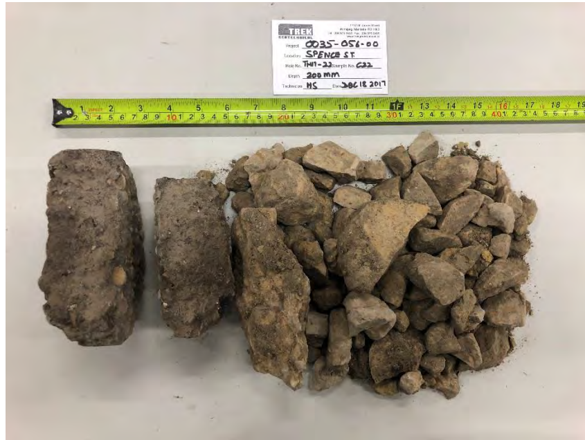
Photo 5: Pavement Core Sample at Test Hole TH17-22
