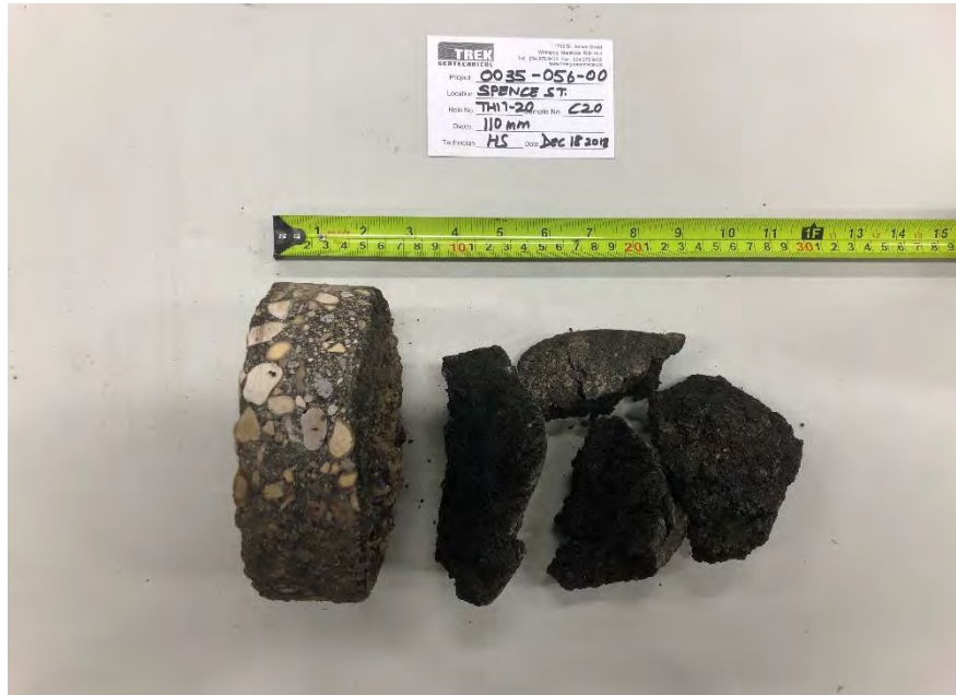
Photo 3: Pavement Core Sample at Test Hole TH17-20
