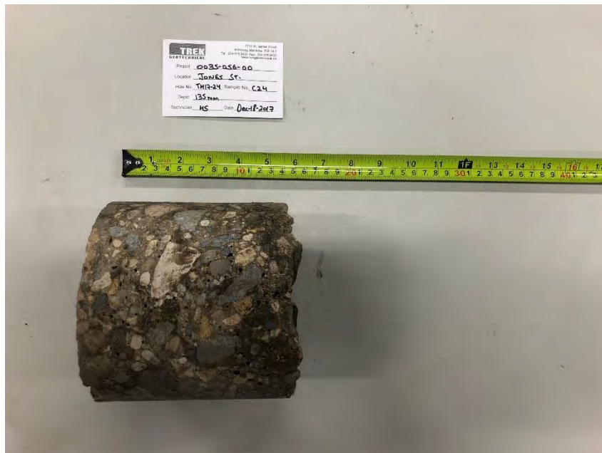
Photo 2: Pavement Core Sample at Test Hole TH17-24
