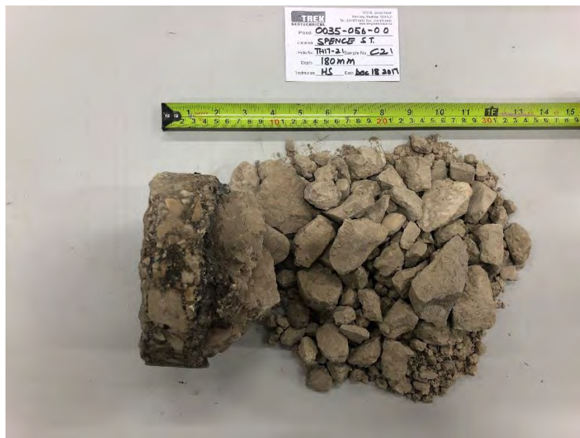
Photo 4: Pavement Core Sample at Test Hole TH17-21
