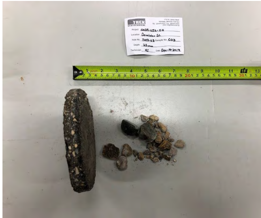
Photo 3: Pavement Core Sample at Test Hole TH17-03 (no recovery of concrete)
