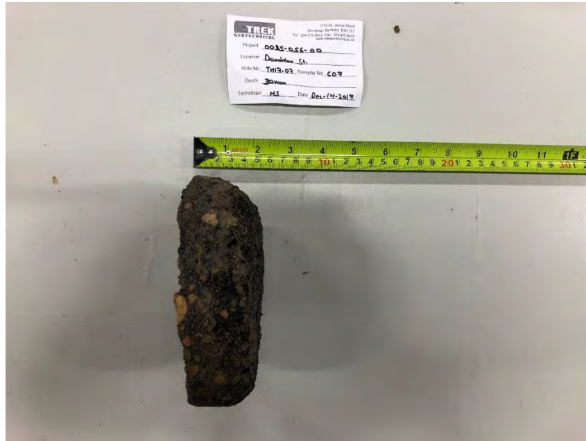
Photo 7: Pavement Core Sample at Test Hole TH17-07 9 (no recovery of concrete)
