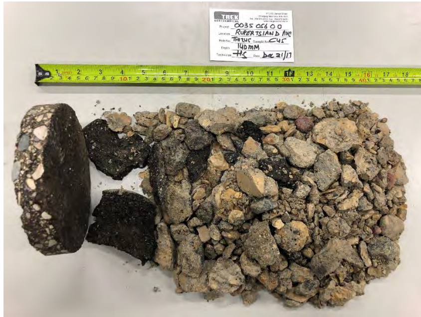
Photo 7: Pavement Core Sample at Test Hole TH17-45
