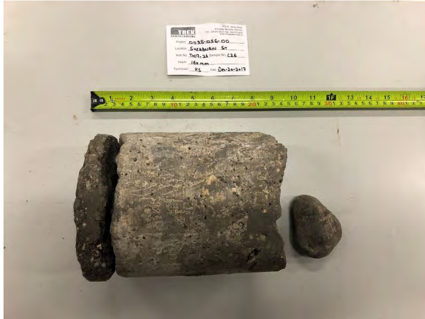
Photo 1: Pavement Core Sample at Test Hole TH17-26
