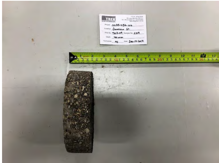
Photo 9: Pavement Core Sample at Test Hole TH17-09 (no recovery of concrete)
