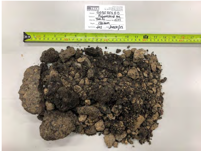
Photo 3: Pavement Core Sample at Test Hole TH17-41
