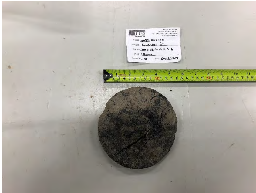
Photo 7: Pavement Core Sample at Test Hole TH17-16 (no recovery of concrete)
