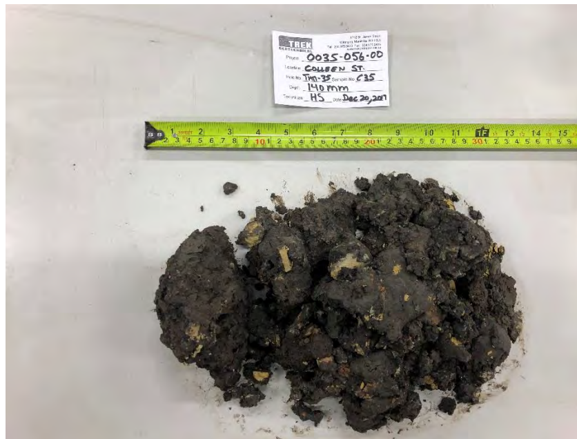
Photo 2: Pavement Core Sample at Test Hole TH17-35
