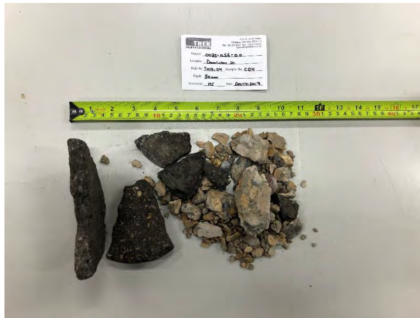
Photo 4: Pavement Core Sample at Test Hole TH17-04
