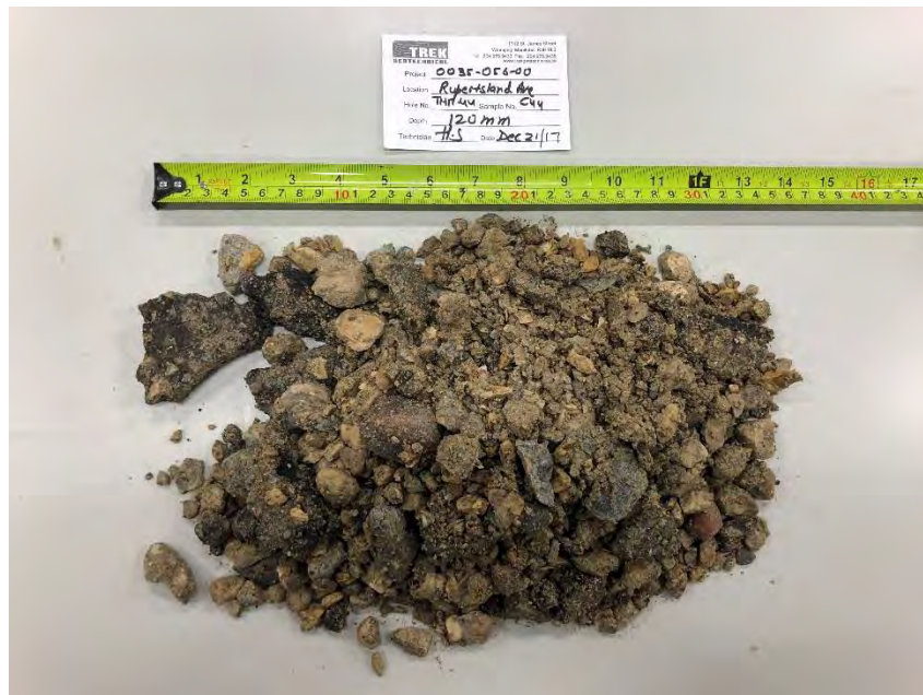
Photo 6: Pavement Core Sample at Test Hole TH17-44
