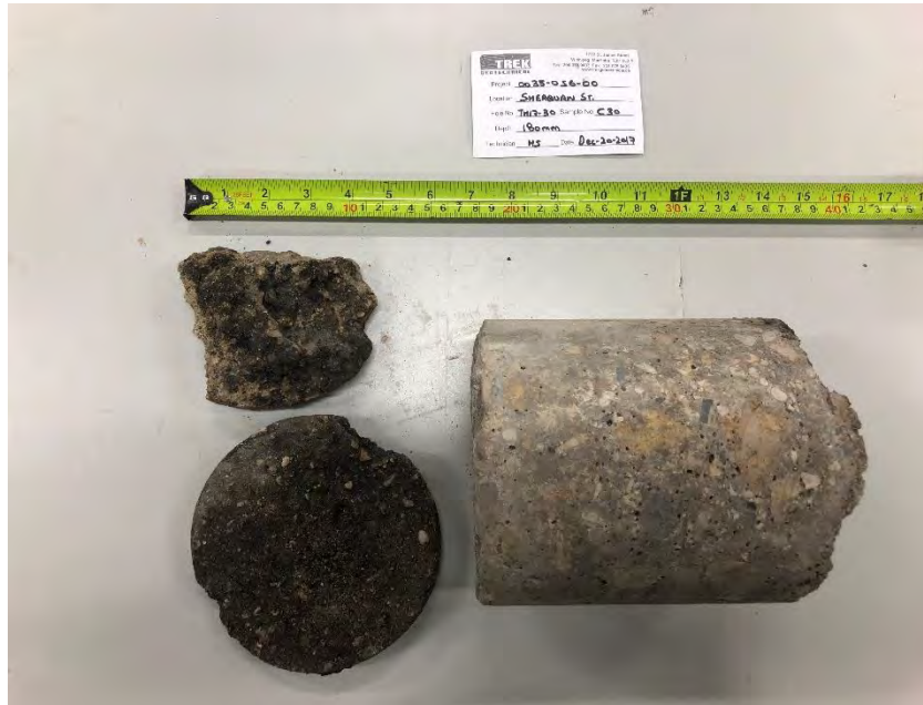
Photo 5: Pavement Core Sample at Test Hole TH17-30
