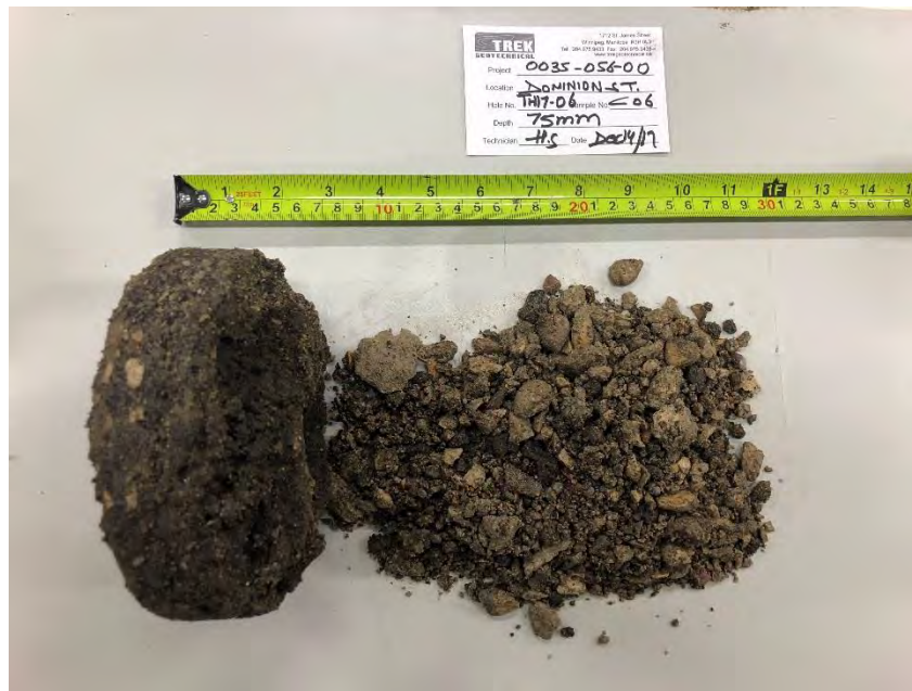
Photo 6: Pavement Core Sample at Test Hole TH17-06
