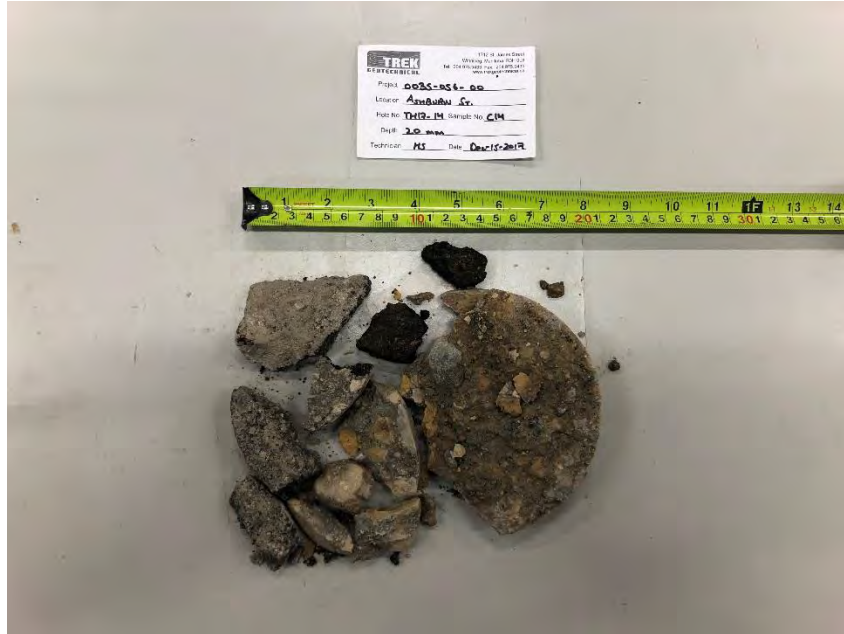
Photo 5: Pavement Core Sample at Test Hole TH17-14
