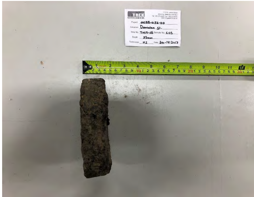
Photo 5: Pavement Core Sample at Test Hole TH17-05 (no recovery of concrete)
