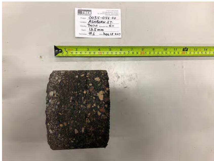
Photo 2: Pavement Core Sample at Test Hole TH17-11 (no recovery of concrete)
