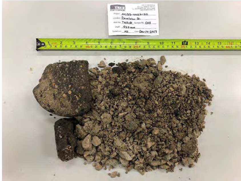
Photo 1: Pavement Core Sample at Test Hole TH17-01
