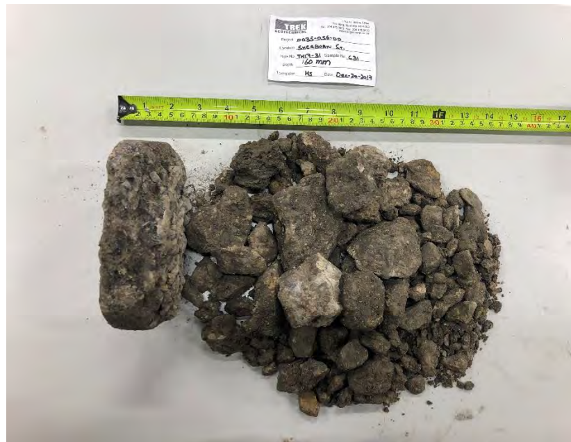
Photo 6: Pavement Core Sample at Test Hole TH17-31
