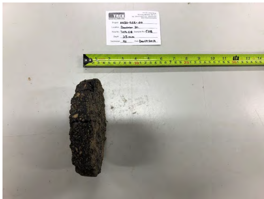
Photo 8: Pavement Core Sample at Test Hole TH17-08 (no recovery of concrete)
