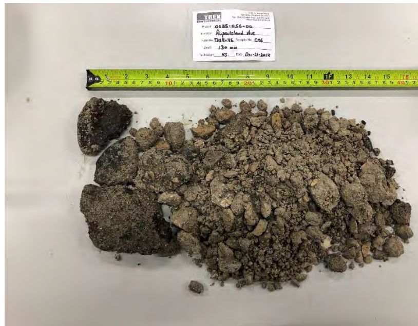
Photo 8: Pavement Core Sample at Test Hole TH17-46
