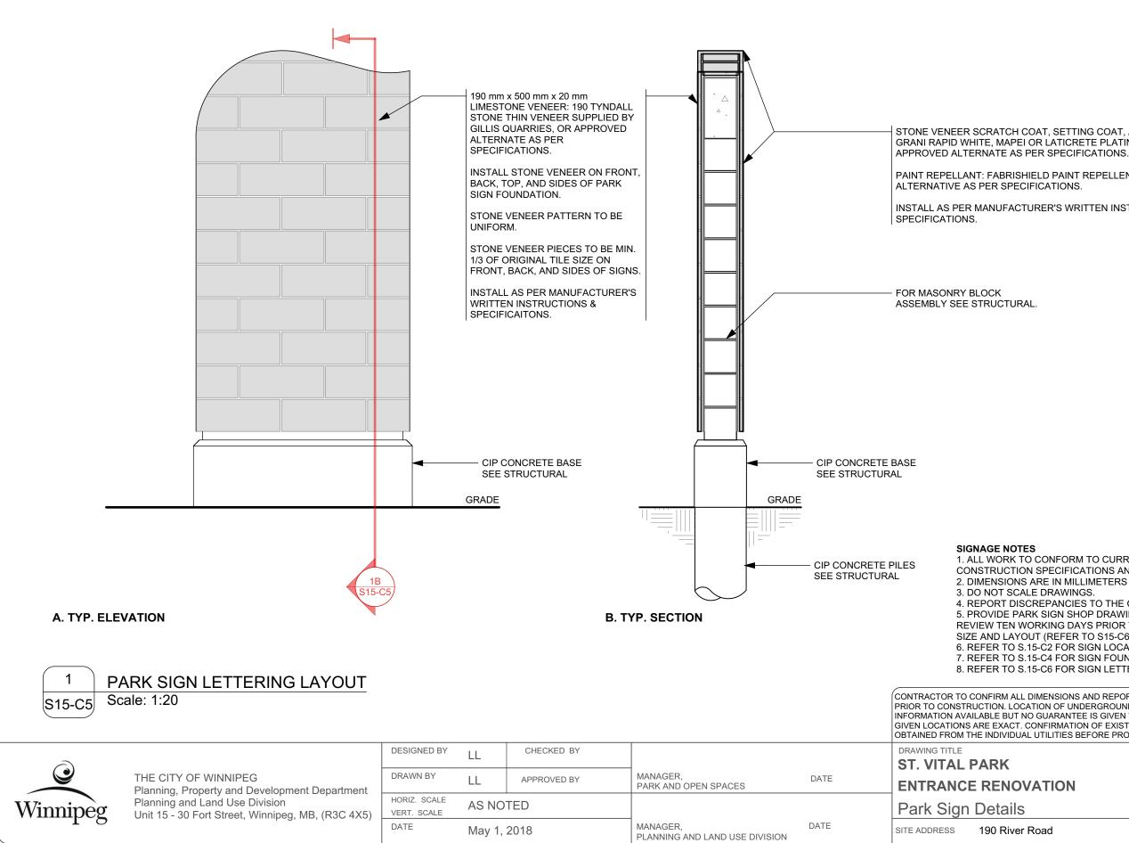
STONE VENEER SCRATCH COAT, SETTING COAT, AND MORTAR/GROUT: GRANI RAPID WHITE, MAPEI OR LATICRETE PLATINUM 254 WHITE, OR
