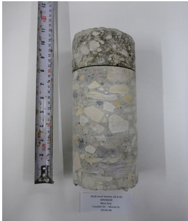
Photograph 17: Pavement Core PC18-18 – Ness Ave
