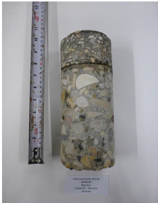
Photograph 18: Pavement Core PC18-19 – Ness Ave
