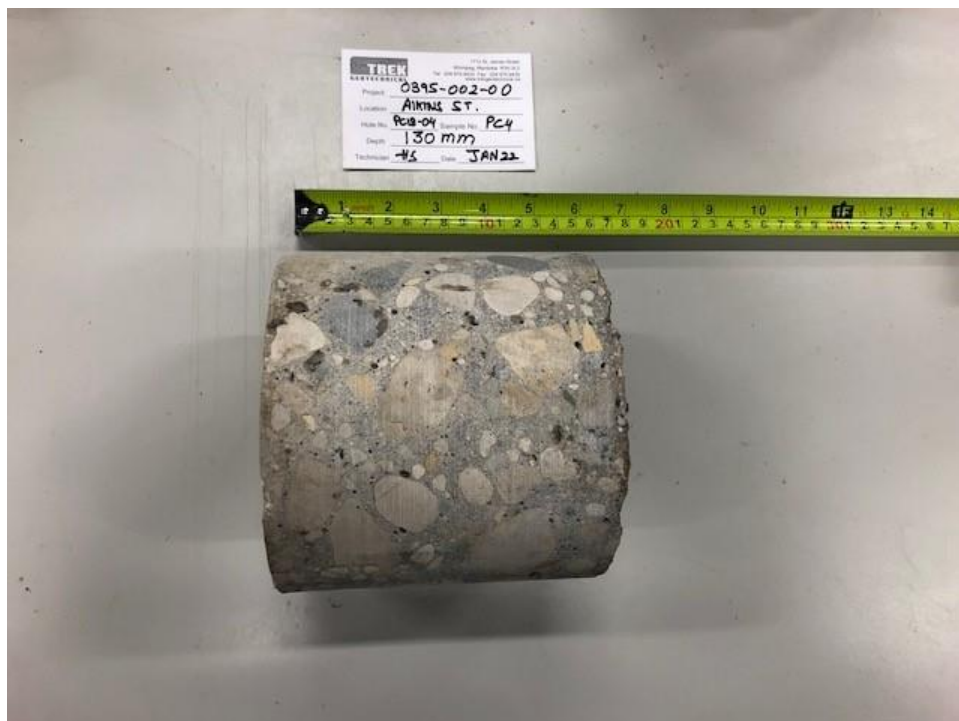
Photo 4: Pavement Core Sample at Test Hole PC18-04
