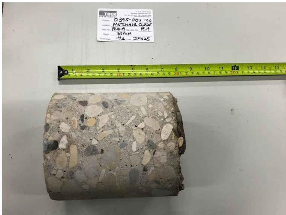
Photo 6: Pavement Core Sample at Test Hole PC18-19
