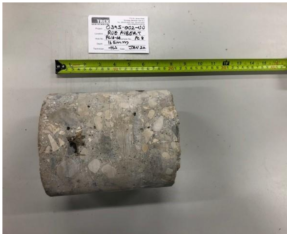
Photo 2: Pavement Core Sample at Test Hole PC18-08
