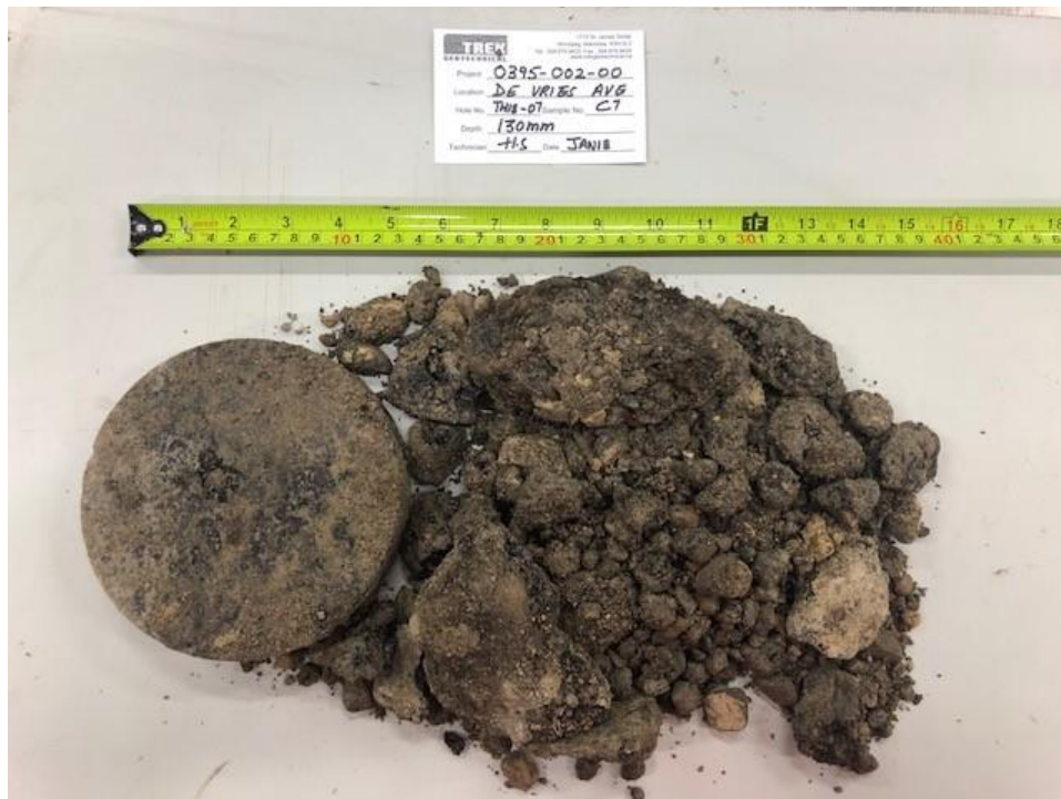
Photo 4: Pavement Core Sample at Test Hole TH18-07
