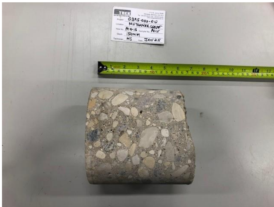
Photo 2: Pavement Core Sample at Test Hole PC18-15
