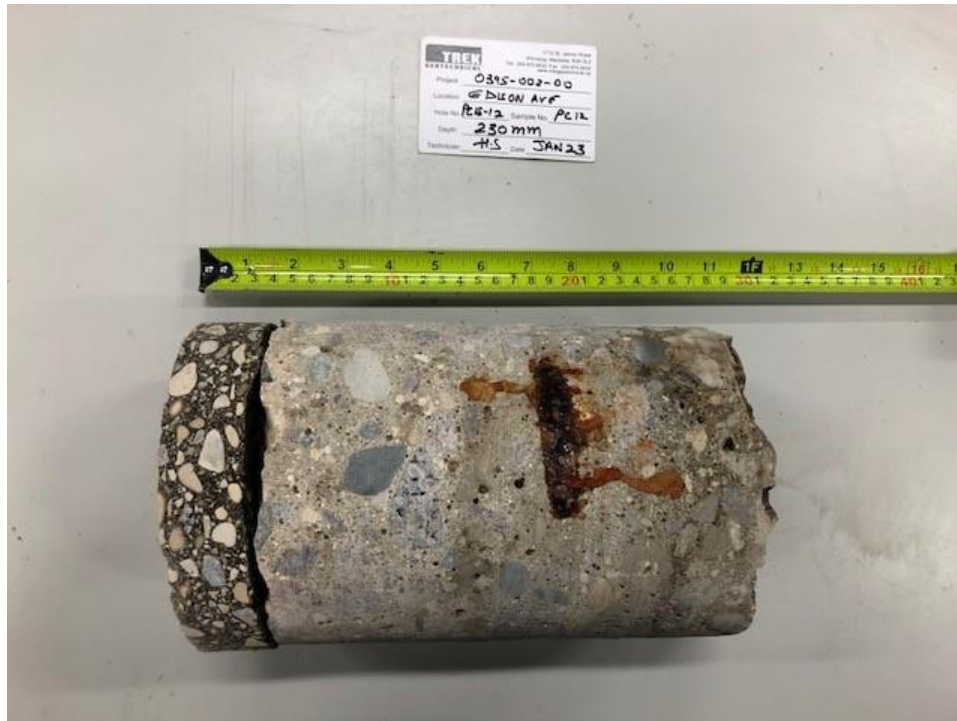
Photo 3: Pavement Core Sample at Test Hole PC18-12
