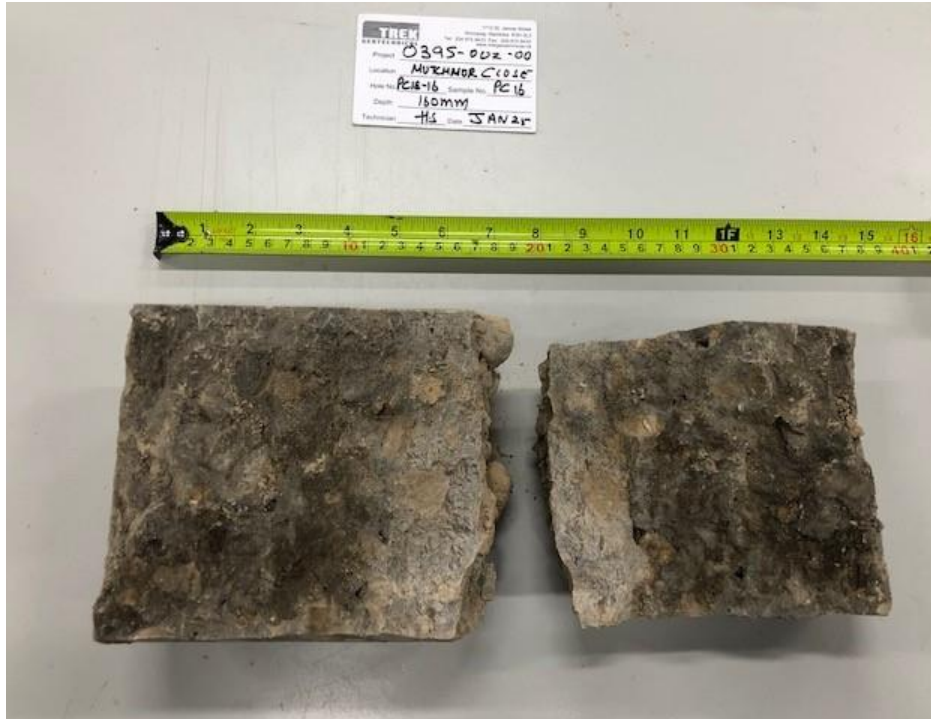
Photo 3: Pavement Core Sample at Test Hole PC18-16
