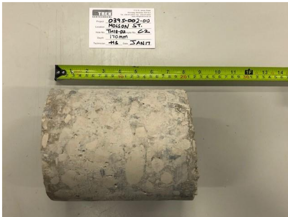
Photo 2: Pavement Core Sample at Test Hole TH18-02
