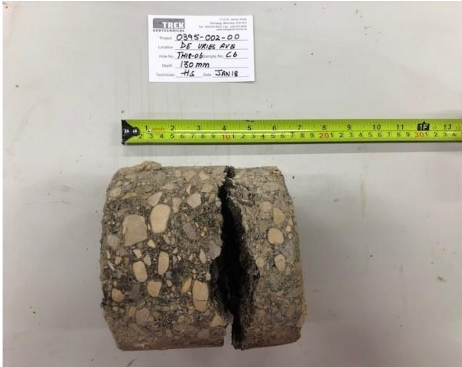
Photo 3: Pavement Core Sample at Test Hole TH18-06
