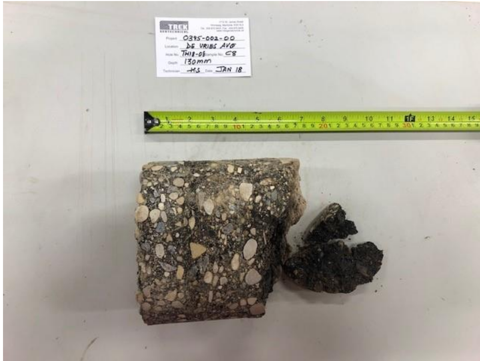
Photo 5: Pavement Core Sample at Test Hole TH18-08
