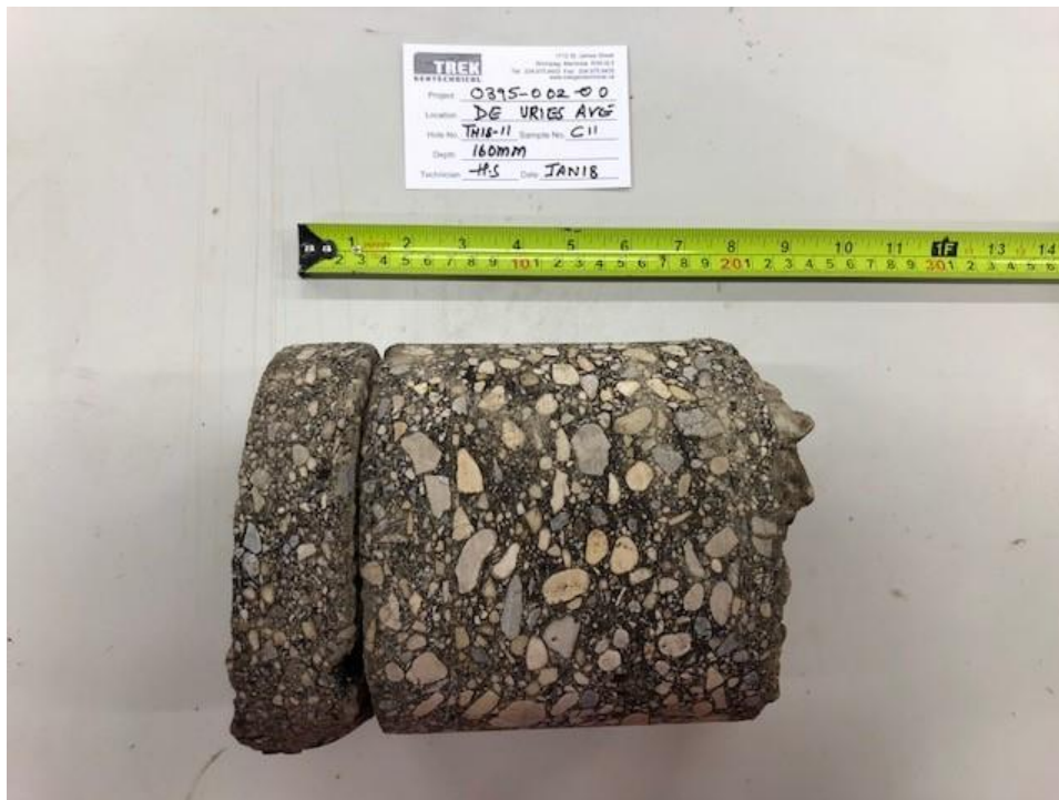
Photo 8: Pavement Core Sample at Test Hole TH18-11
