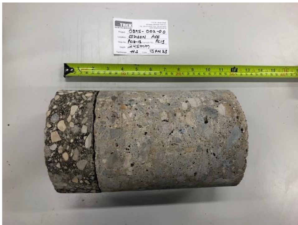
Photo 4: Pavement Core Sample at Test Hole PC18-13
