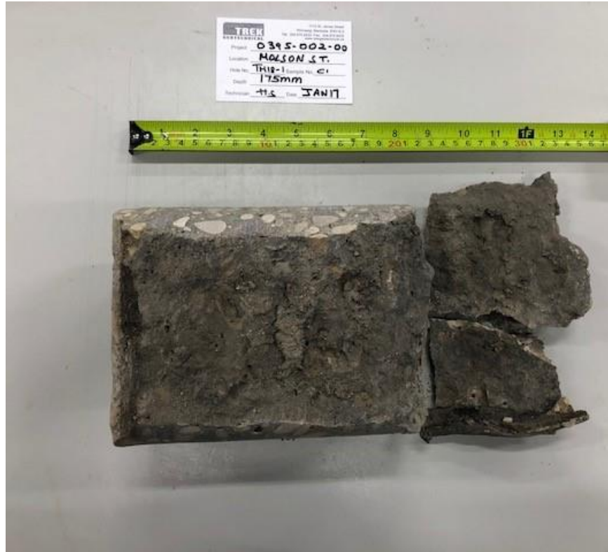
Photo 1: Pavement Core Sample at Test Hole TH18-01
