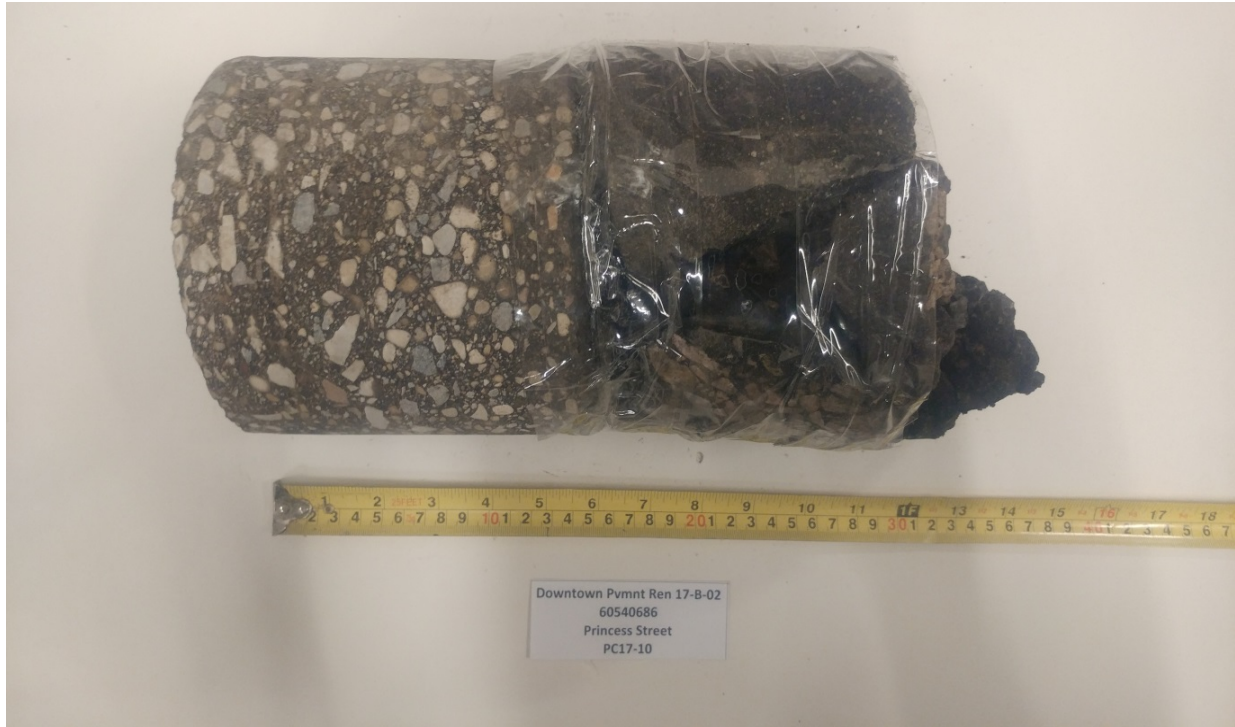
Photograph 11: Pavement Core PC17-10 – Princess Street
