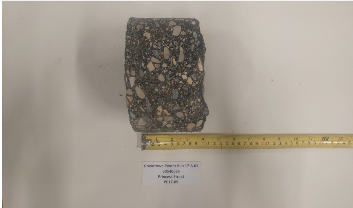
Photograph 9: Pavement Core PC17-09 – Princess Street
