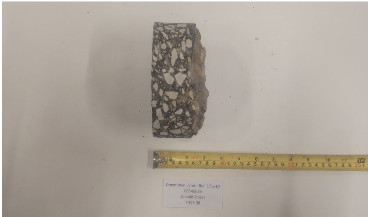
Photograph 8: Test Hole TH17-08 – Donald Street
