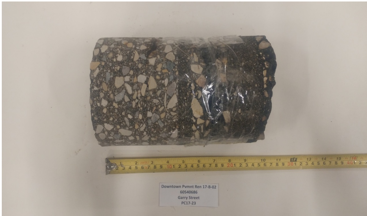
Photograph 24: Pavement Core PC17-23 – Garry Street
