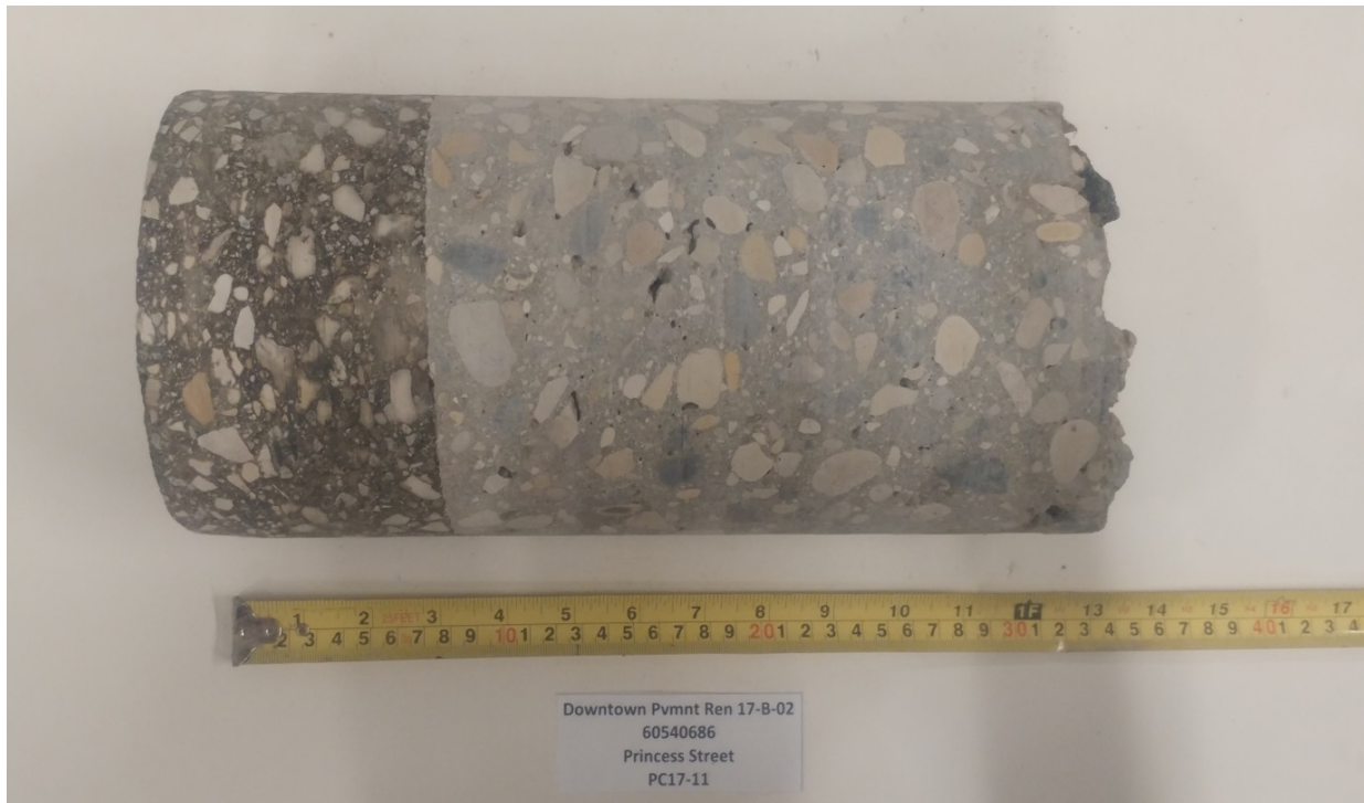
Photograph 12: Pavement Core PC17-11 – Princess Street
