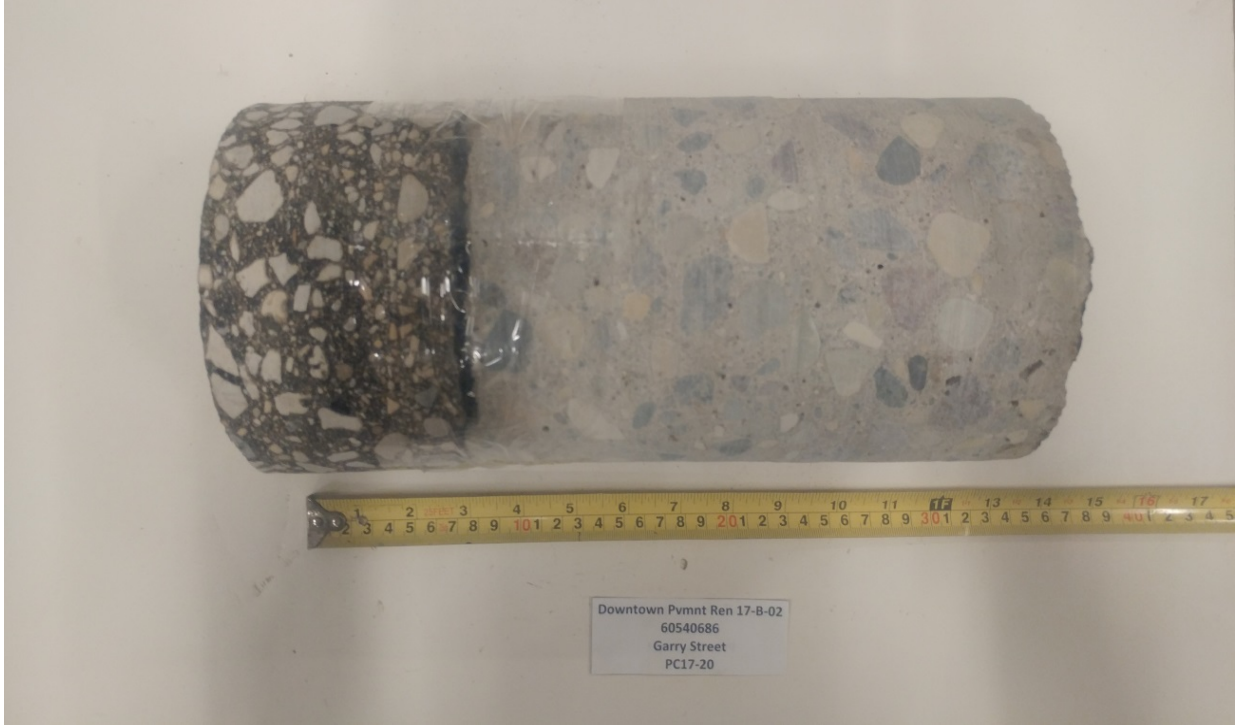
Photograph 21: Pavement Core PC17-20 – Garry Street
