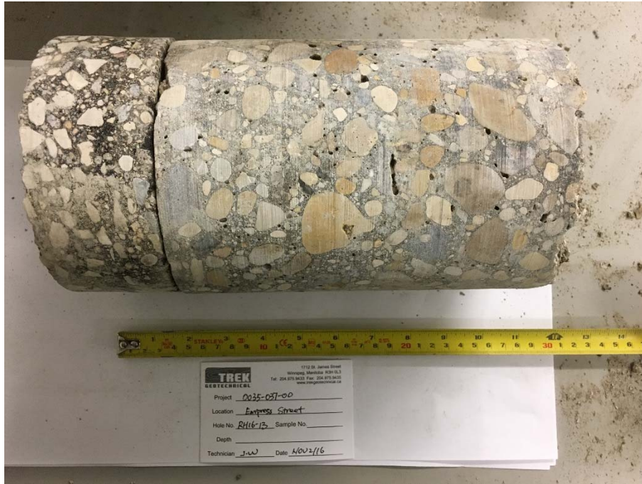
Photo 11: Pavement Core Sample at Test Hole RH16-13
