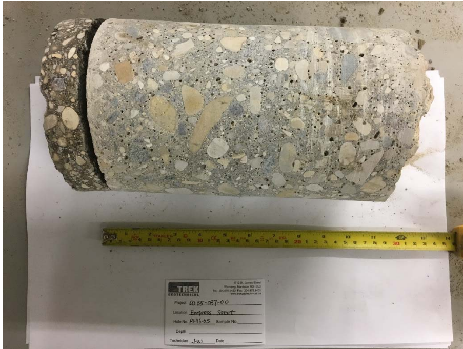
Photo 3: Pavement Core Sample at Test Hole RH16-05
