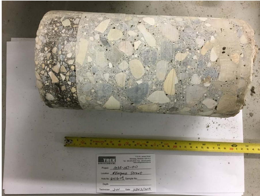
Photo 7: Pavement Core Sample at Test Hole RH16-09
