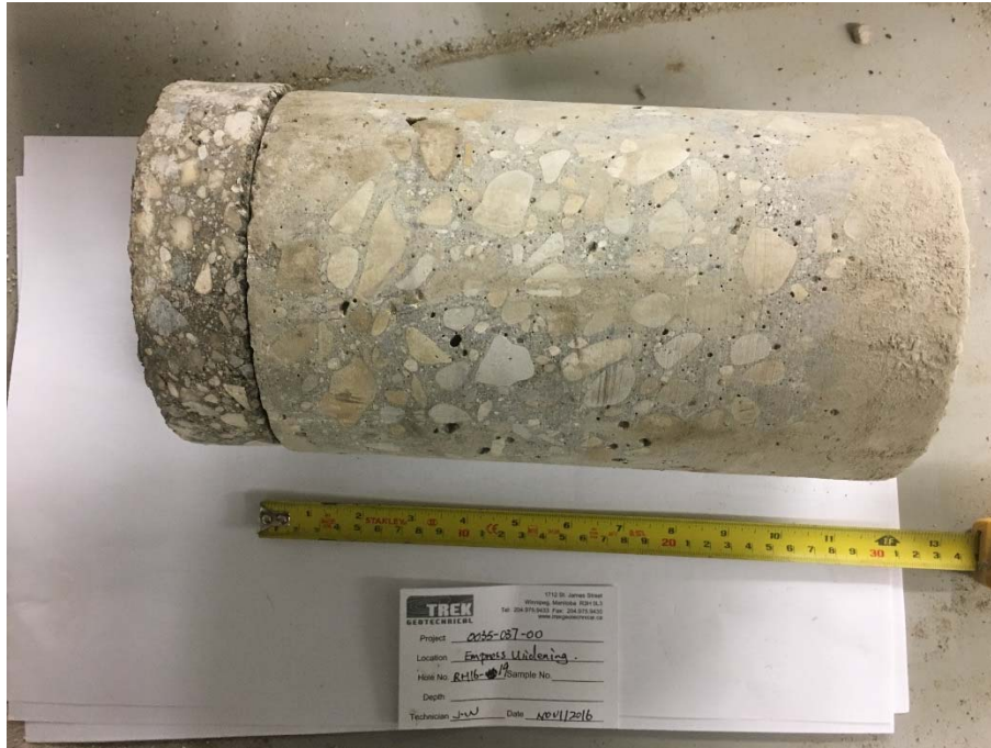
Photo 17: Pavement Core Sample at Test Hole RH16-19
