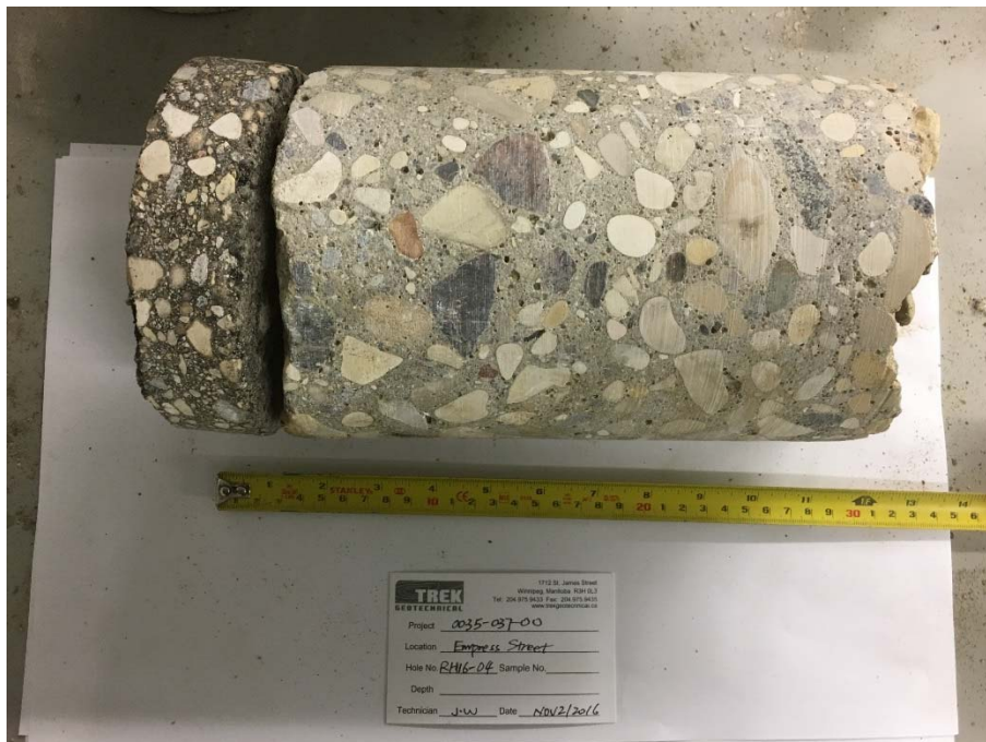
Photo 2: Pavement Core Sample at Test Hole RH16-04
