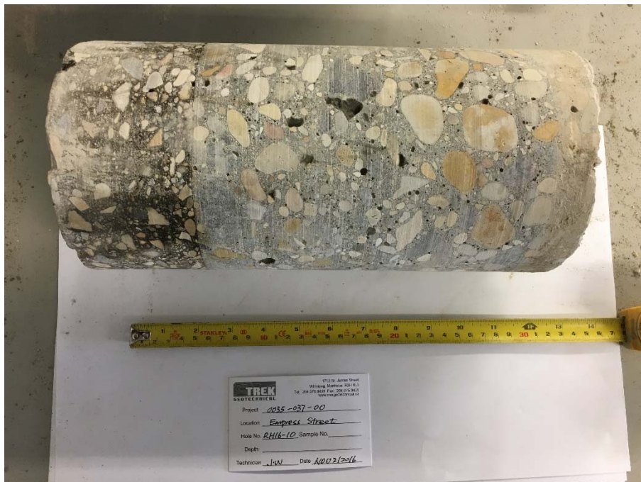
Photo 8: Pavement Core Sample at Test Hole RH16-10
