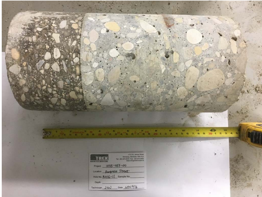
Photo 9: Pavement Core Sample at Test Hole RH16-11
