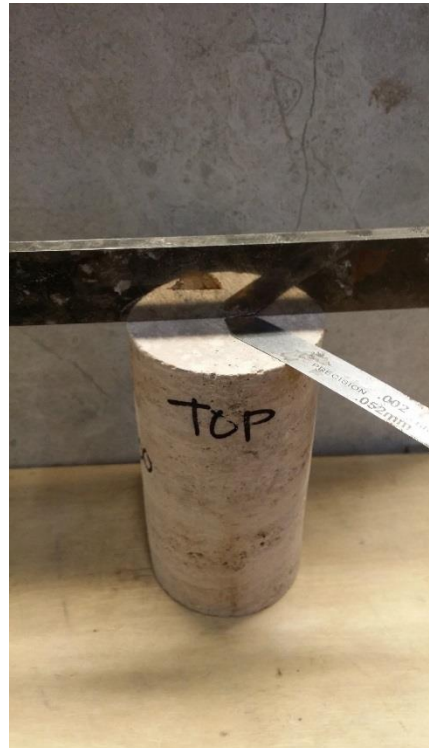
Photo 2: Top of Core Sample before Break
