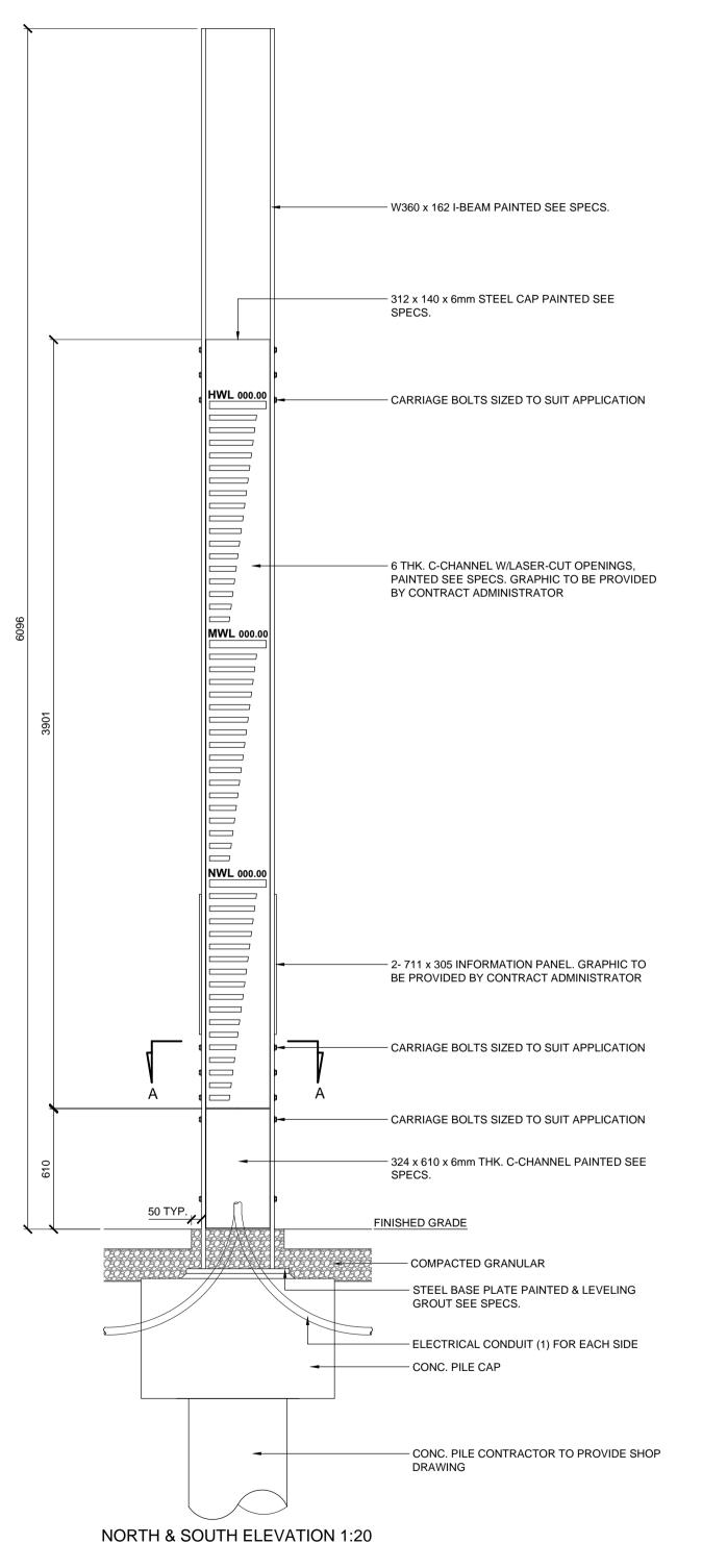
1. CONTRACTOR TO PROVIDE SHOP DRAWINGS FOR WATER LEVEL INDICATOR INCLUDING FOUNDATION AND STEEL COMPONENTS. SHOP DRAWINGS TO BE SEALED BY ENGINEER SEE SPECS. 2. FOUNDATION DESIGN BY CONTRACTOR. CONTRACTOR TO SUBMIT SHOP DRAWINGS SEALED BY
