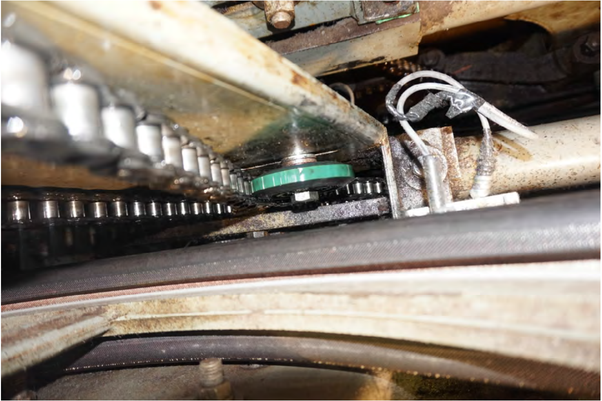
This is the new, non-aluminium, handrail drive chain tensioner.
