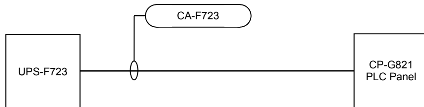
Figure 7-3: Instrument Cable Identification Example – Identified Equipment
