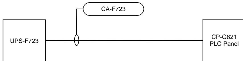
Figure 7-2: Instrument Cable Identification Example – Identified Equipment
