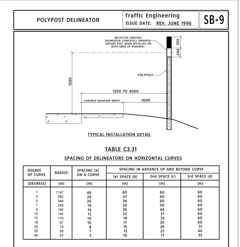
NOTE:(a) SPACING ON CURVE= $2x \sqrt{0.3R}$  WHERE R= RADIUS IN METRES.
