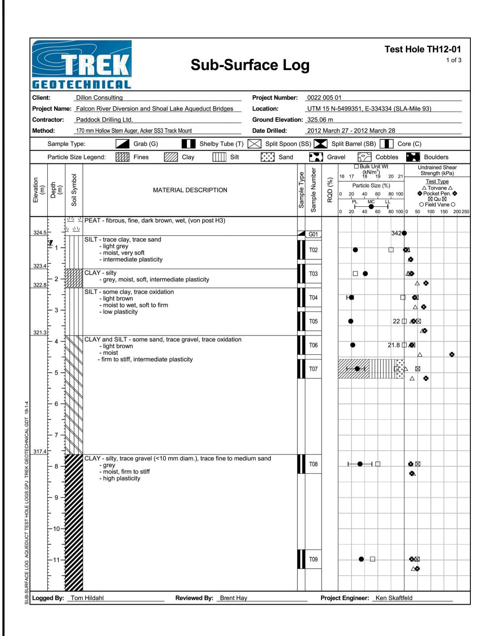
BORE HOLE NO. 1 (1 OF 3) TREK TEST HOLE TH12-01
