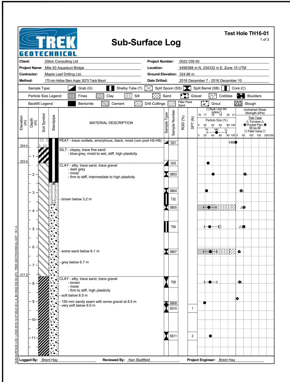
BORE HOLE NO. 1 (1 OF 3) TREK TEST HOLE TH16-01
