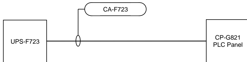
Figure 7-3: Instrument Cable Identification Example – Identified Equipment
