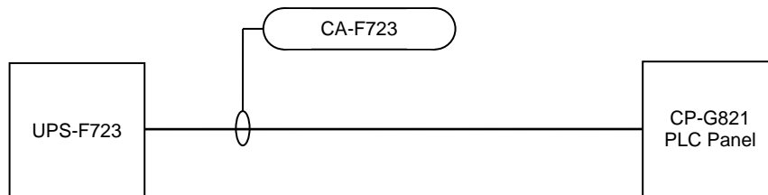
Figure 7-3: Instrument Cable Identification Example – Identified Equipment
