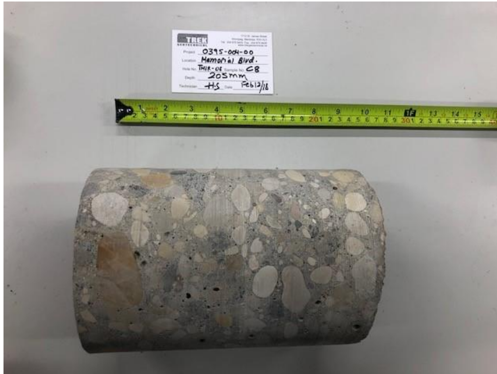
Photo 6: Pavement Core Sample at Test Hole TH18-08
