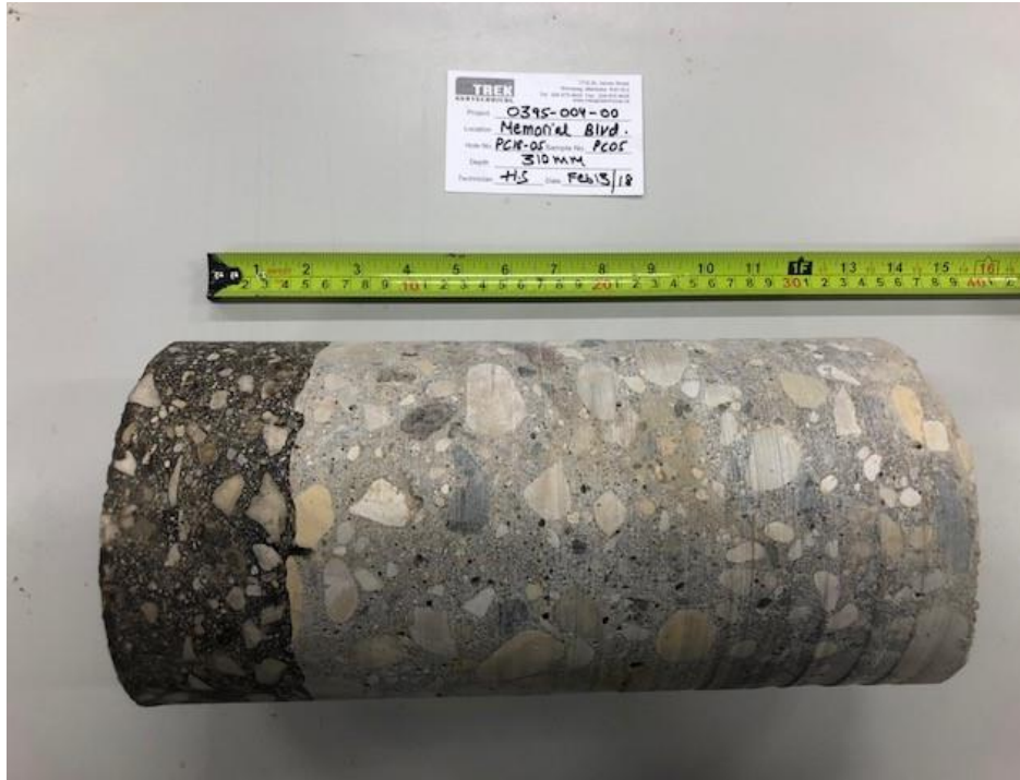
Photo 5: Pavement Core Sample at Pavement Hole PC18-05
