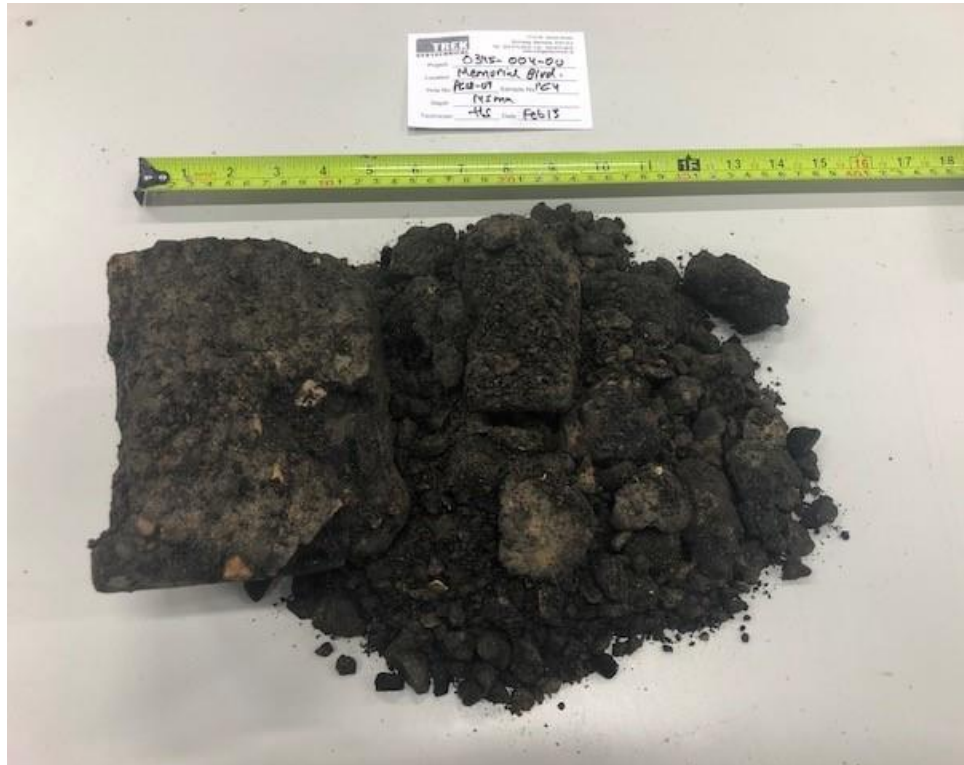
Photo 4: Pavement Core Sample at Pavement Hole PC18-04
