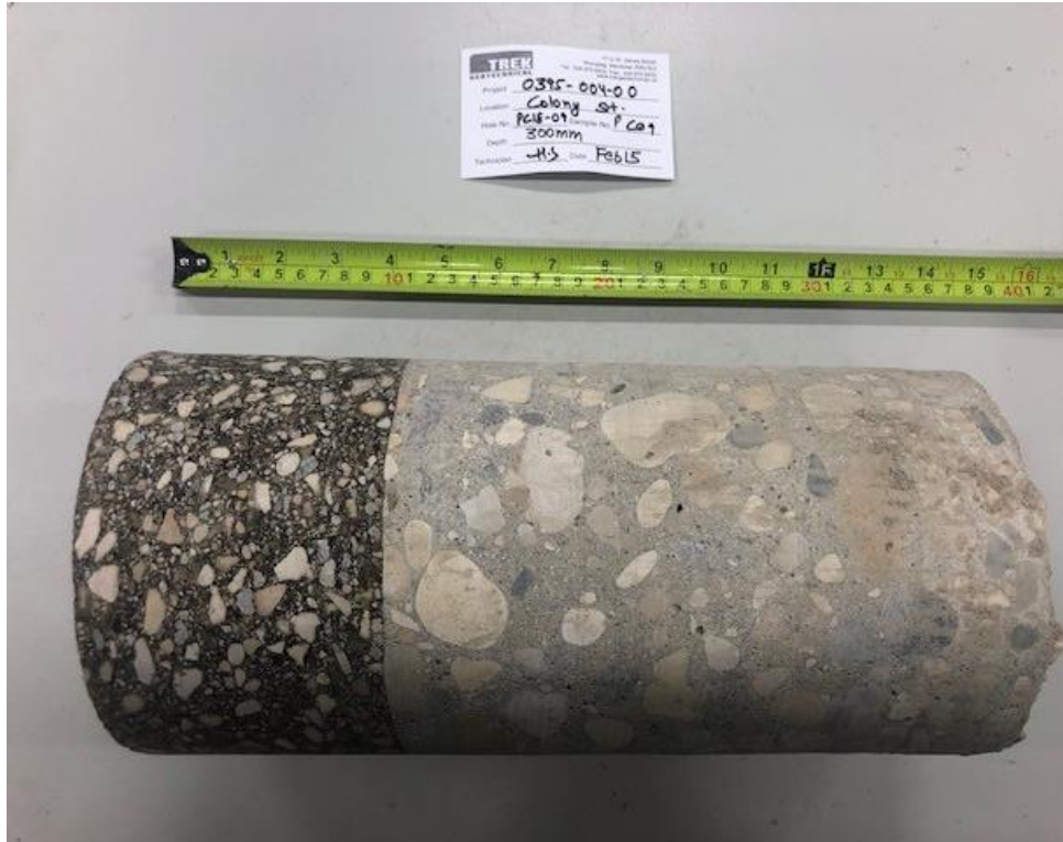
Photo 3: Pavement Core Sample at Pavement Hole PC18-09
