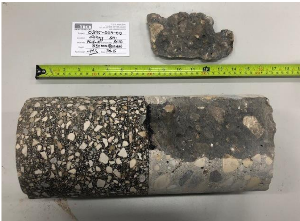
Photo 4: Pavement Core Sample at Pavement Hole PC18-10
