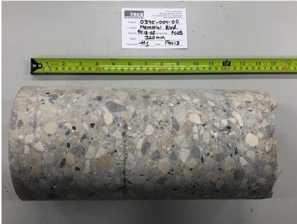
Photo 3: Pavement Core Sample at Pavement Hole PC18-03
