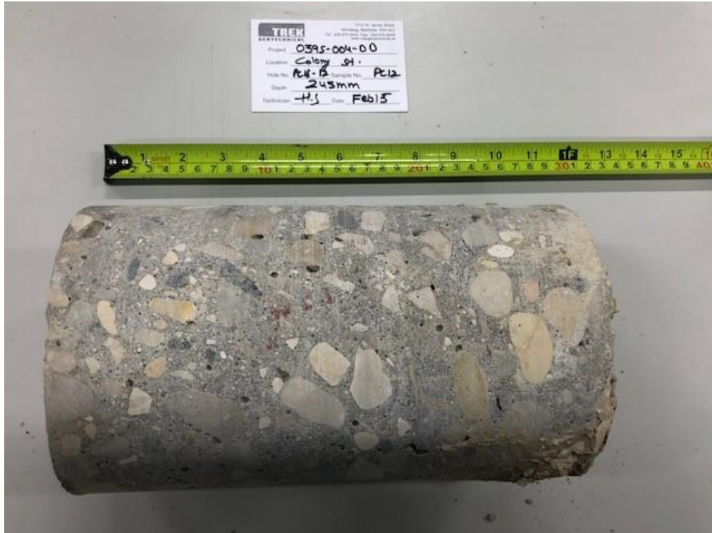
Photo 6: Pavement Core Sample at Pavement Hole PC18-12
