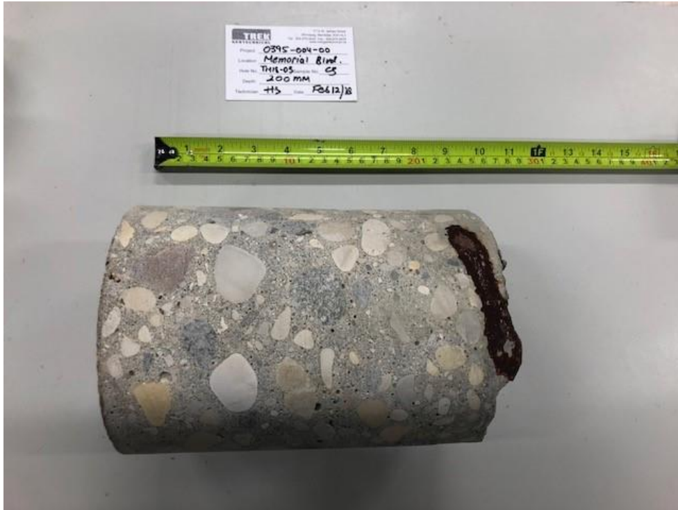
Photo 1: Pavement Core Sample at Test Hole TH18-03
