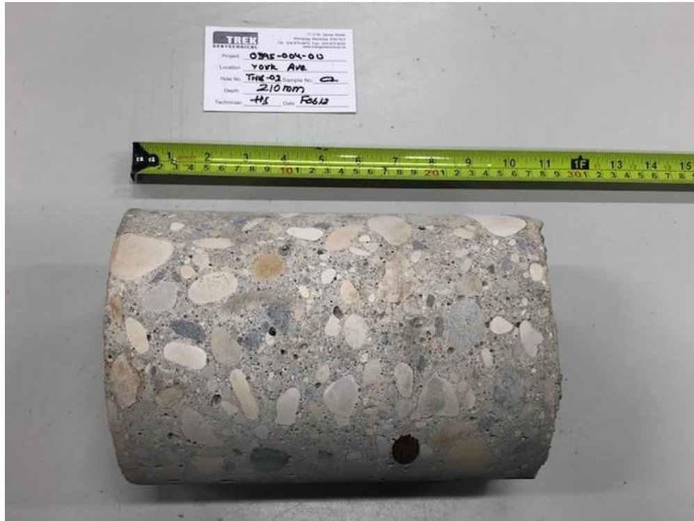
Photo 2: Pavement Core Sample at Test Hole TH18-02
