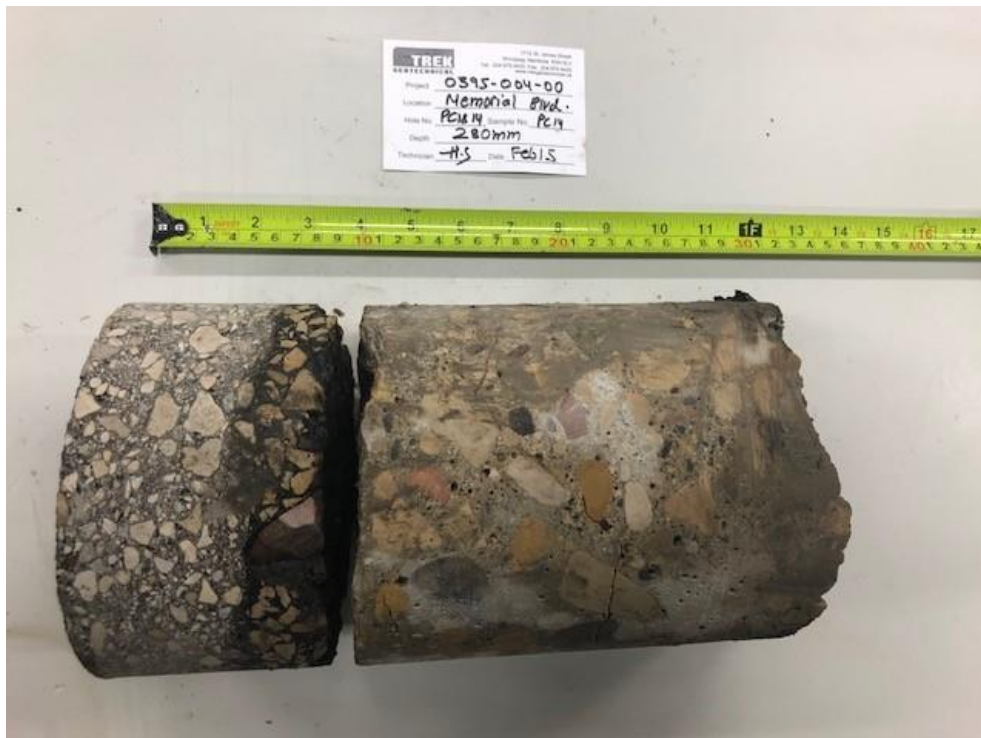
Photo 8: Pavement Core Sample at Pavement Hole PC18-14
