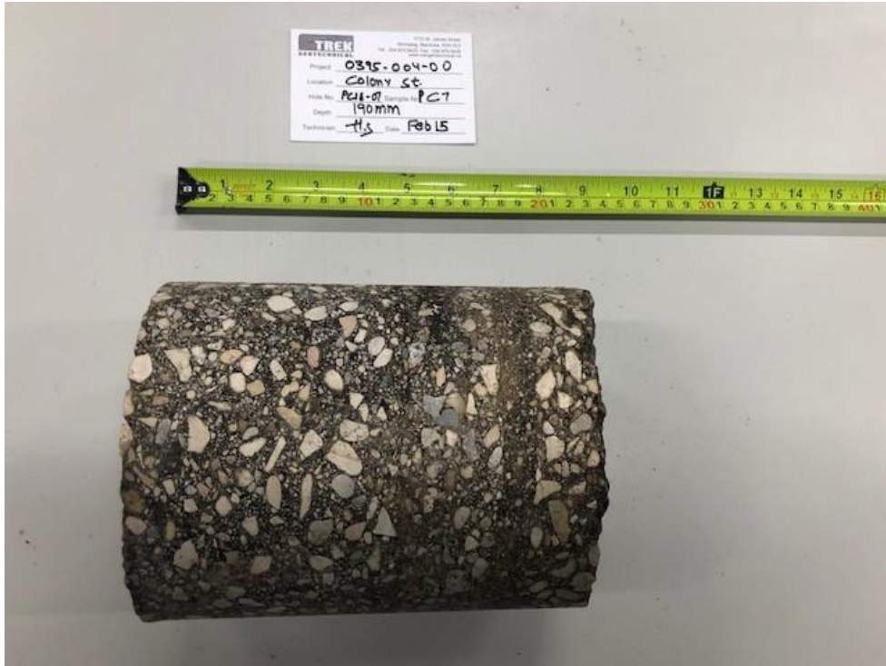
Photo 1: Pavement Core Sample at Pavement Hole PC18-07
