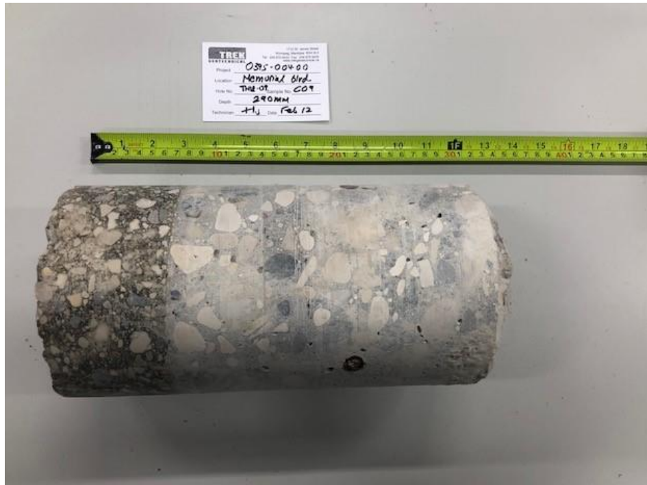
Photo 7: Pavement Core Sample at Test Hole TH18-09
