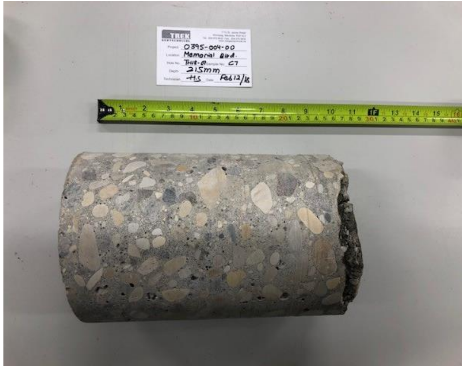
Photo 5: Pavement Core Sample at Test Hole TH18-07
