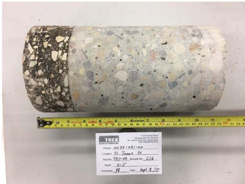
Photo 5: Pavement Core Sample at Test Hole TH17-05
