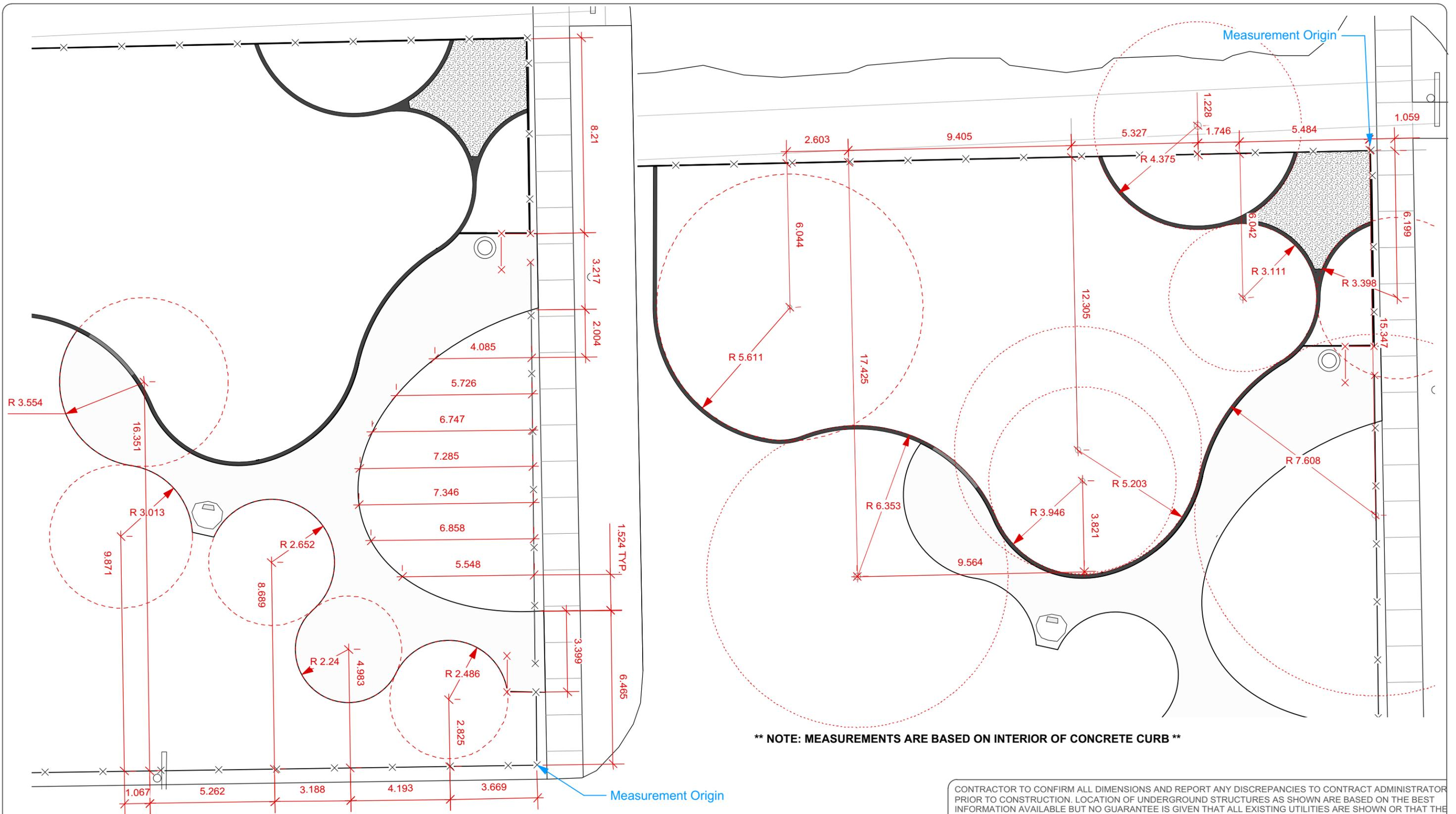
**\*\* NOTE: MEASUREMENTS ARE BASED ON INTERIOR OF CONCRETE CURB \*\***
