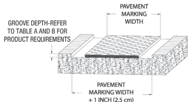
Figure 1 – Groove and Pavement Marking – Typical Section
