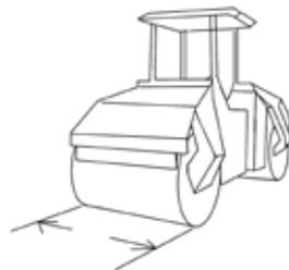
Under normal conditions, a minimum of three passes of the finishing roller is required to hot inlay the tape. **An inlay is considered successful when approximately 50 to 60 percent of the tape's thickness is below the asphalt surface.** (See Figure 1 on page 4.) To test for embedment use a 40 mil depth gauge or a bridge micrometer. For more information on embedment, contact technical service at 1-800-553-1380.
