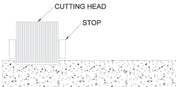
**Figure 2 - Initial Pass, Intersection Groove Cut**
