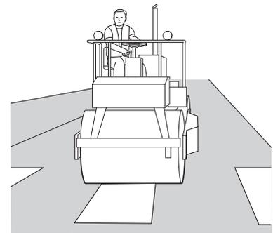
Under normal conditions, a minimum of three passes back and forth of the finishing roller are required to hot inlay the tape. **An inlay is considered successful when approximately 50 to 60 percent of the tape's thickness is below the asphalt surface.** (See Figure 1 on page 4). **To test for embedment use a 40 mil depth gauge or a bridge micrometer. For more information on embedment, contact technical service at 1-800-553-1380.**
