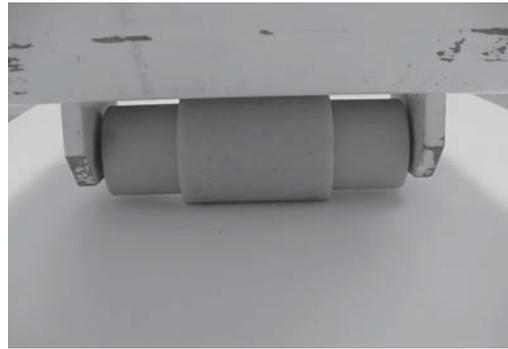
Figure 11 – Tamper cart roller cut for groove tamping
