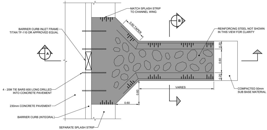
**REINFORCED CONCRETE SPILLWAY WITH RIPRAP (TYPICAL WITH CURB INLET FRAME)**
