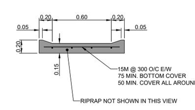
**CROSS SECTION B - THROUGH SPILLWAY**
