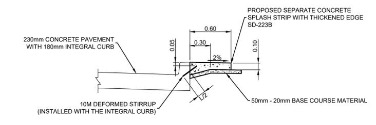
**SEPARATE CONCRETE SPLASH STRIP WITH THICKENED EDGE**
