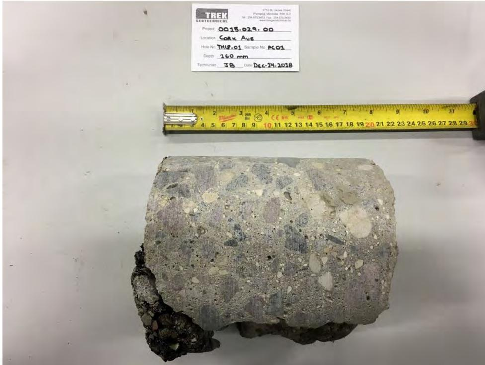
Photo 1: Pavement Core Sample at Test Hole TH18-01
