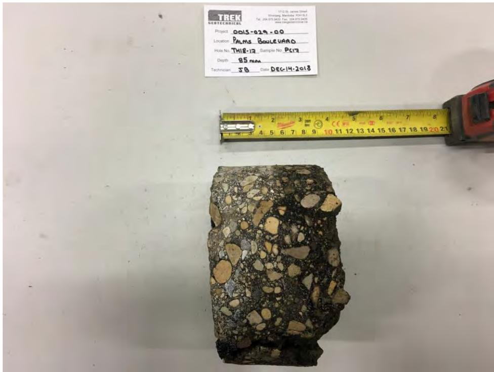
Photo 2: Pavement Core Sample at Test Hole TH18-17
