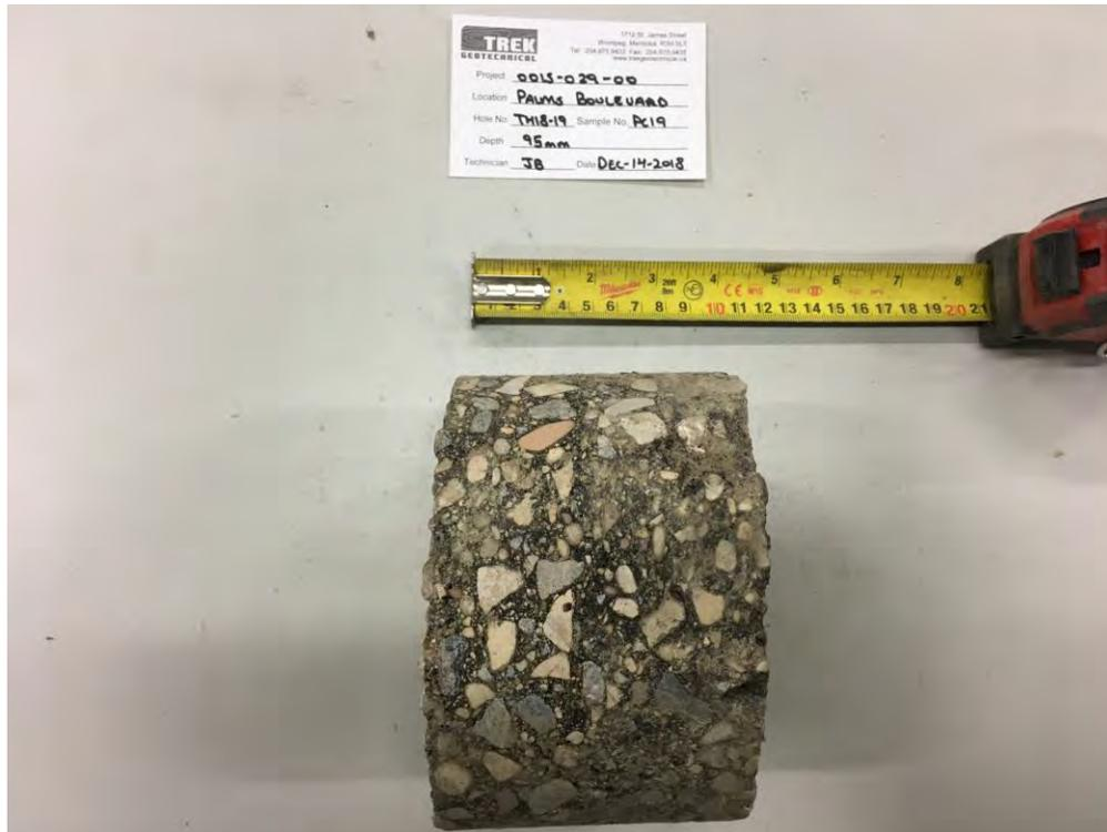
Photo 5: Pavement Core Sample at Test Hole TH18-19
