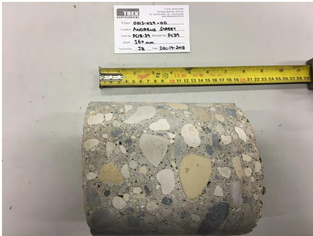
Photo 10: Pavement Core Sample at Test Hole PC18-39
