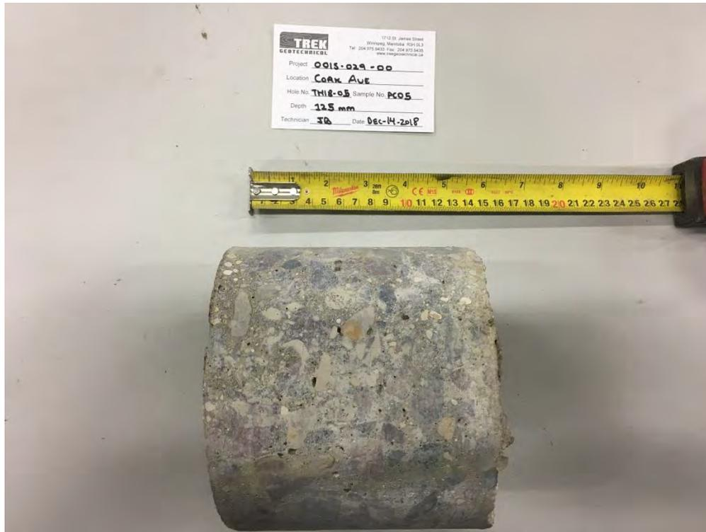
Photo 5: Pavement Core Sample at Test Hole TH18-05
