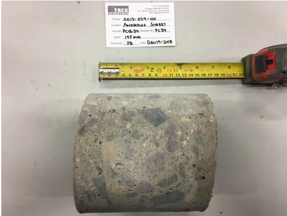
Photo 5: Pavement Core Sample at Test Hole PC18-34
