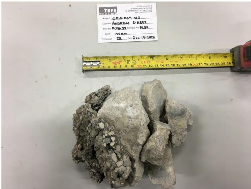
Photo 8: Pavement Core Sample at Test Hole PC18-37
