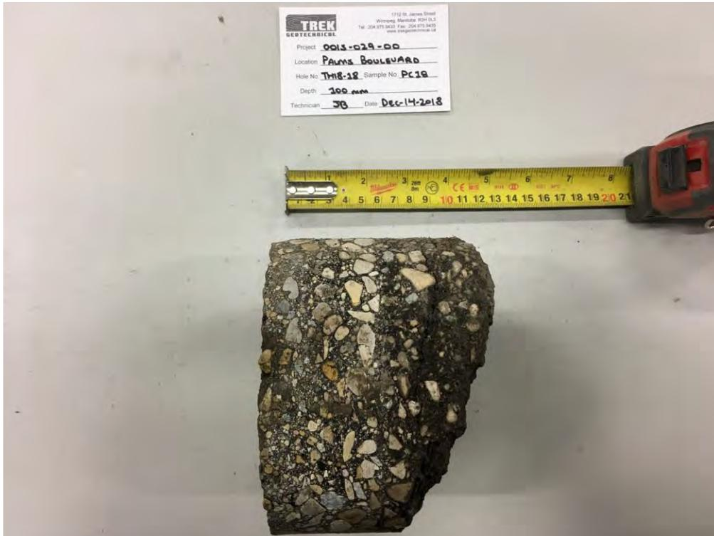
Photo 4: Pavement Core Sample at Test Hole TH18-18
