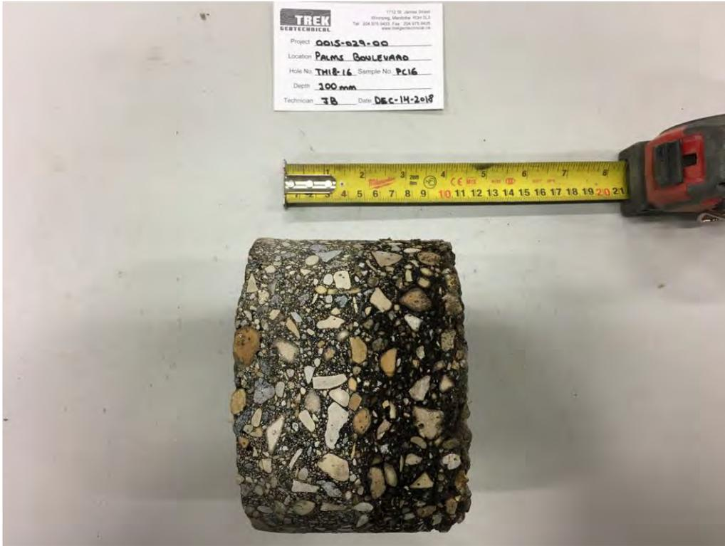
Photo 1: Pavement Core Sample at Test Hole TH18-16
