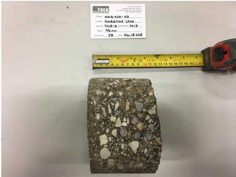
Photo 3: Pavement Core Sample at Test Hole TH18-13
