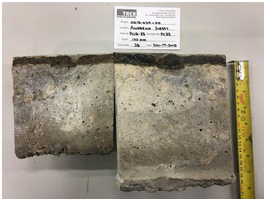
Photo 4: Pavement Core Sample view of Joint at Test Hole PC18-33
