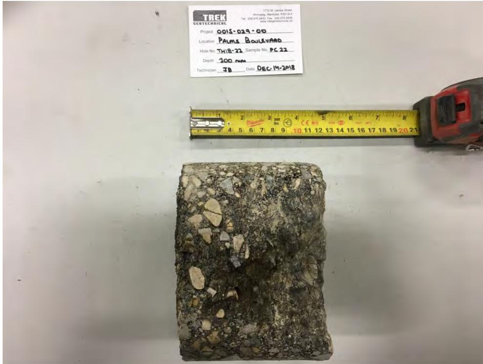
Photo 3: Pavement Core Sample at Test Hole TH18-22
