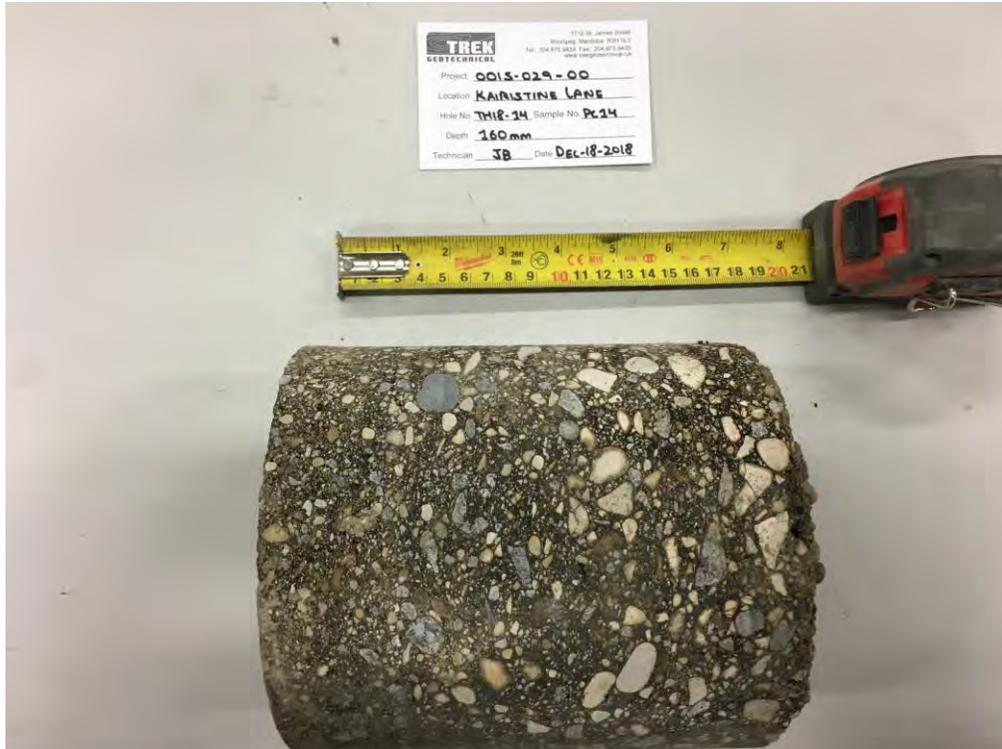
Photo 4: Pavement Core Sample at Test Hole TH18-14
