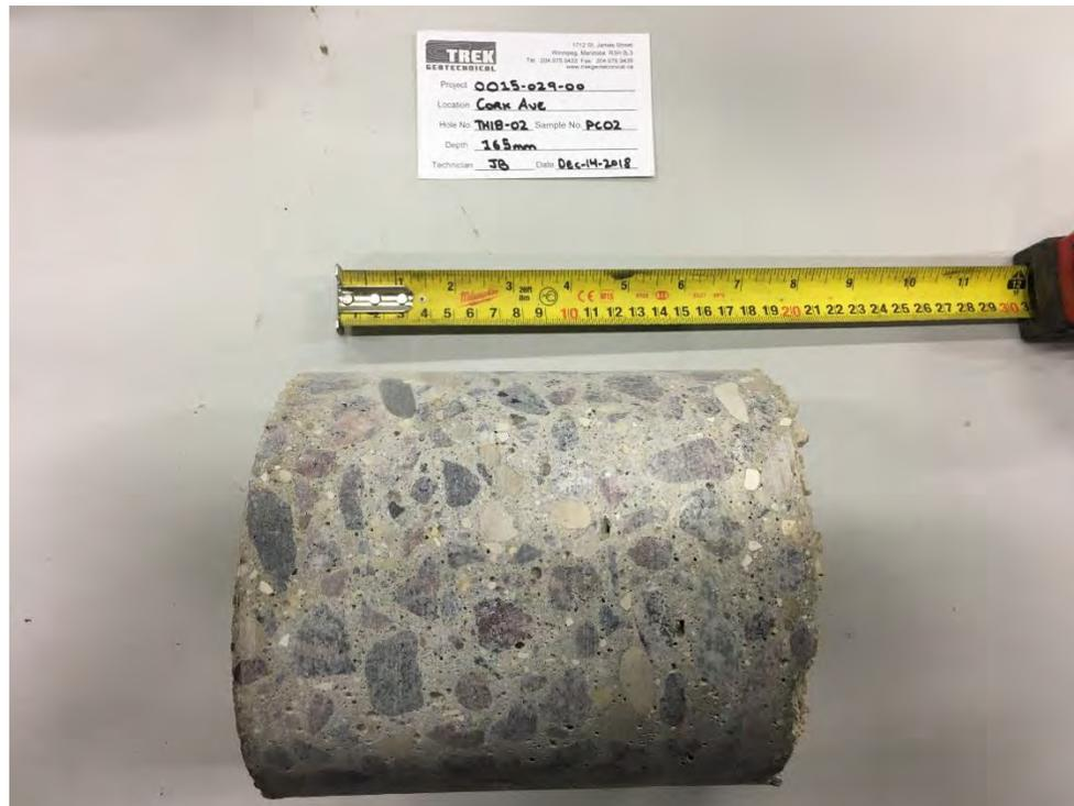
Photo 2: Pavement Core Sample at Test Hole TH18-02
