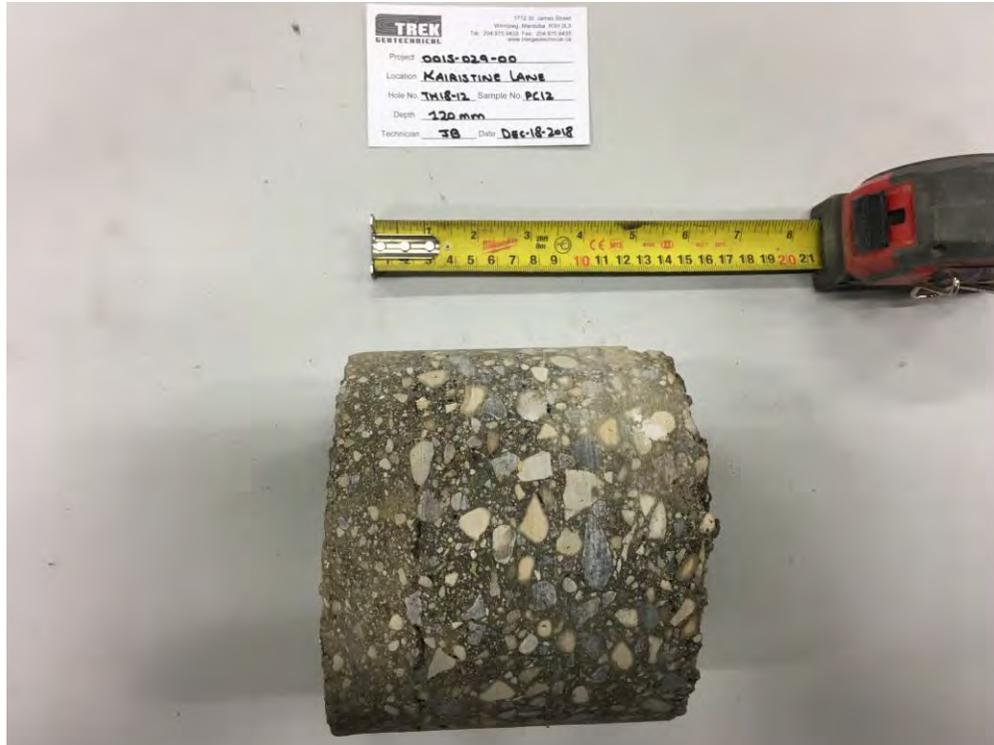
Photo 2: Pavement Core Sample at Test Hole TH18-12
