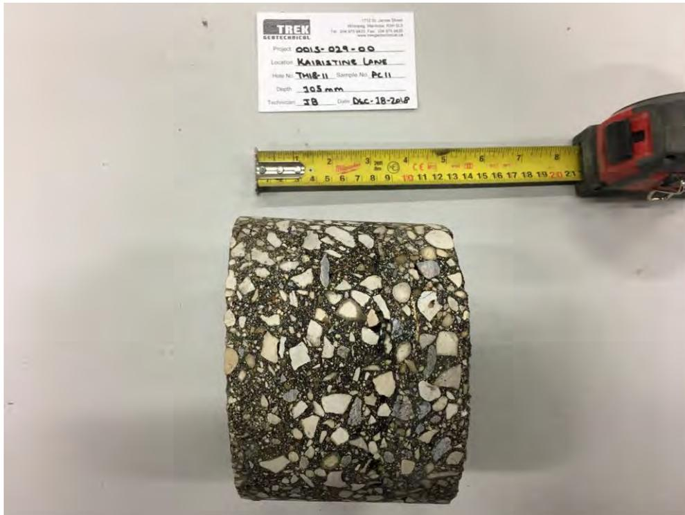
Photo 1: Pavement Core Sample at Test Hole TH18-11
