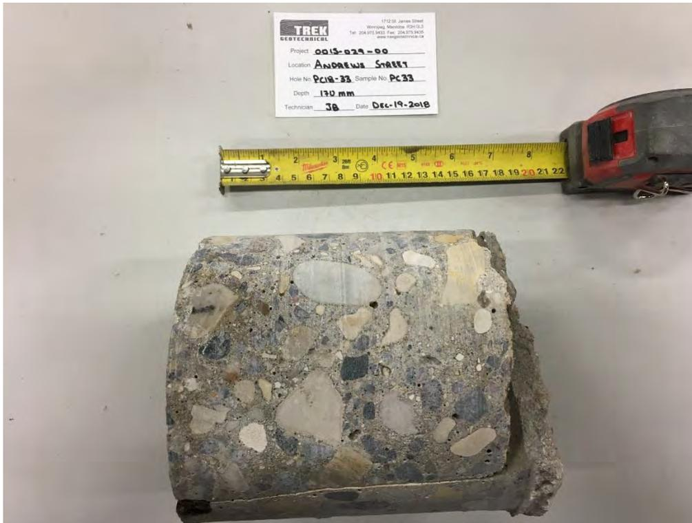
Photo 3: Pavement Core Sample at Test Hole PC18-33 (On Joint)
