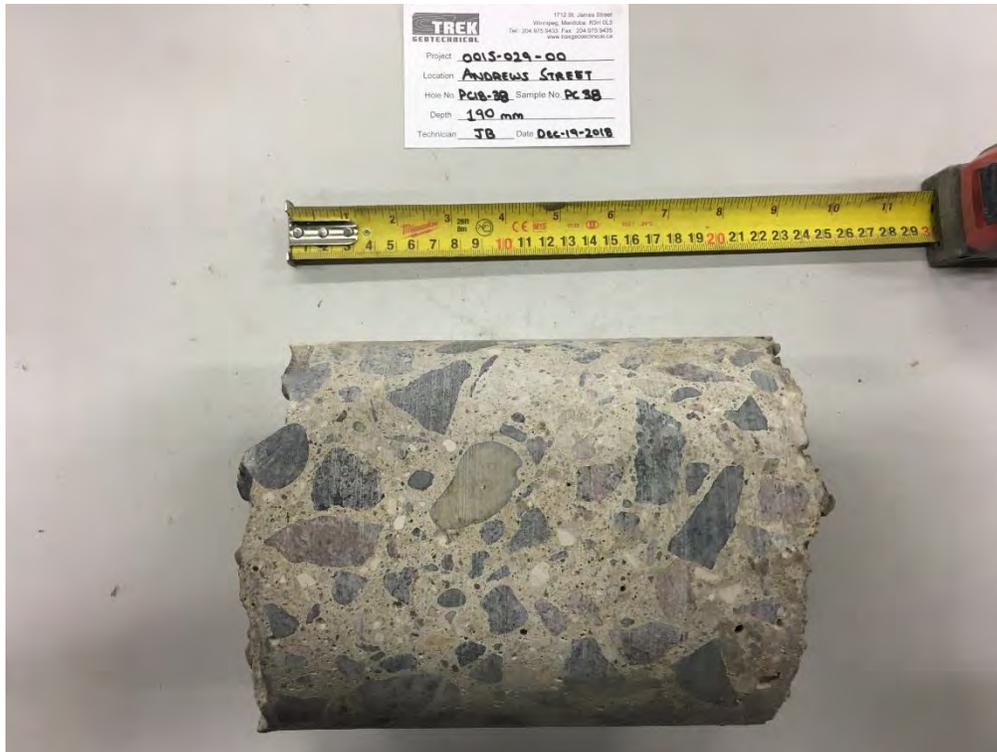
Photo 9: Pavement Core Sample at Test Hole PC18-38
