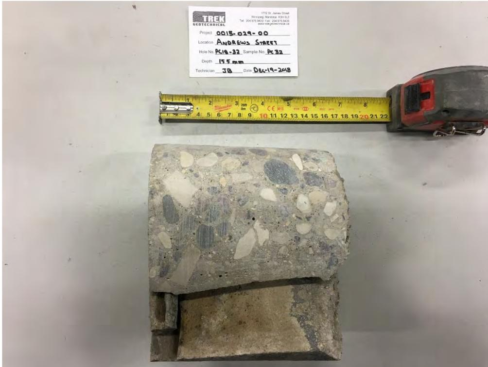
Photo 1: Pavement Core Sample at Test Hole PC18-32 (On Joint)
