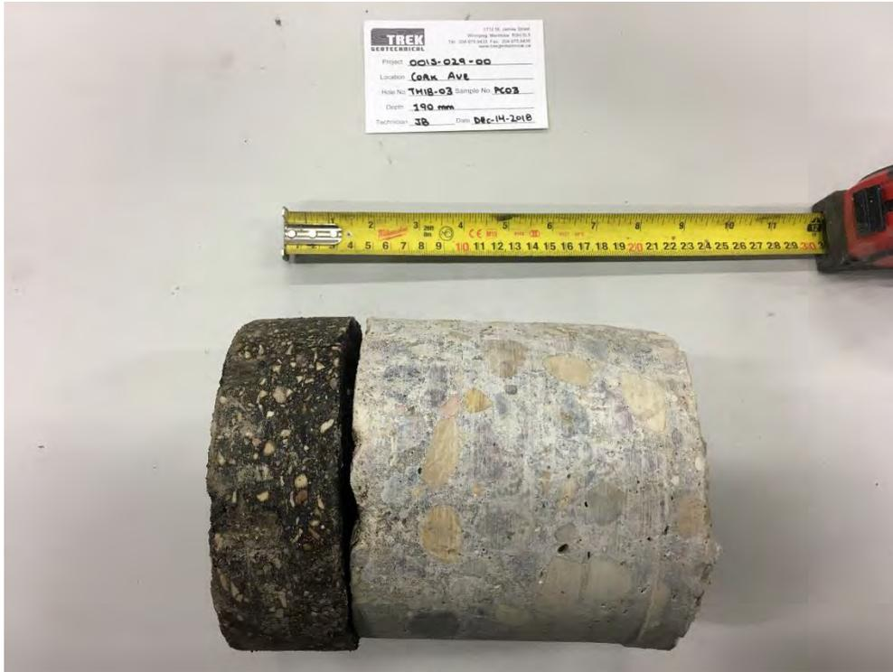
Photo 3: Pavement Core Sample at Test Hole TH18-03
