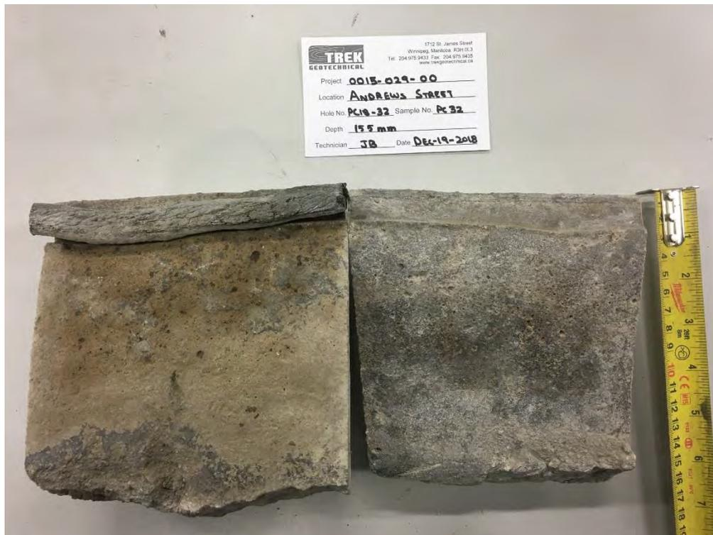
Photo 2: Pavement Core Sample view of Joint at Test Hole PC18-32
