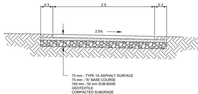
**75 mm ASPHALT PATH TYPICAL CROSS SECTION**
