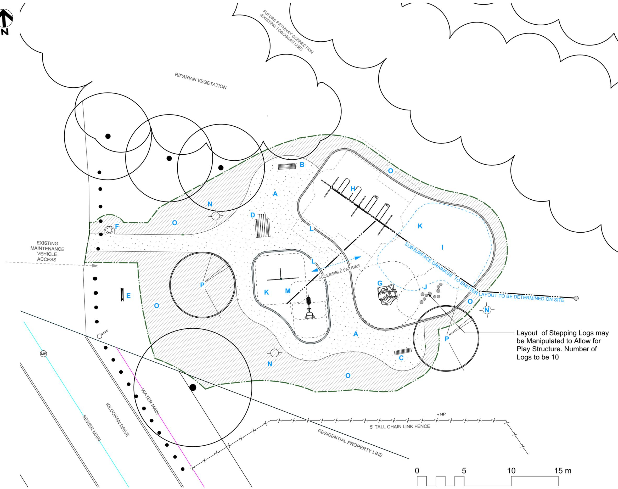
Layout of Stepping Logs may be Manipulated to Allow for Play Structure. Number of Logs to be 10
