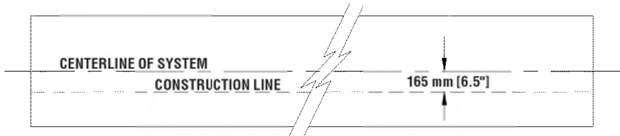
Figure 16 (Top view of concrete foundation)
