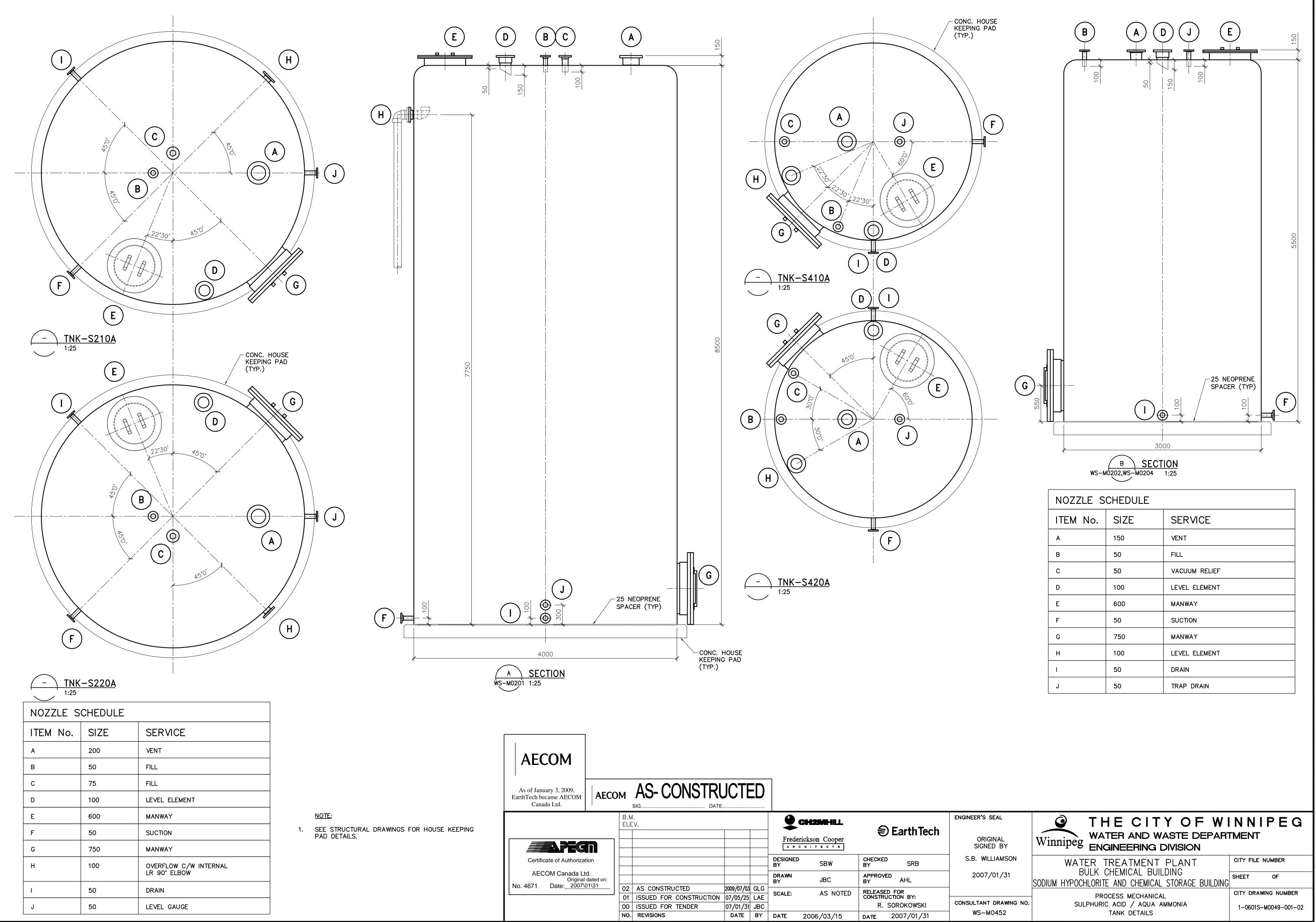
L:\WORK\79000\79538\02A-CAD\ALL\SUBMISSION\AS BUILT RECORD\C40 - 792-2006 BULK CHEM & HYPOCHL BLDG\PROCESS\BULK CHEMICAL\AS CONSTRUCTED DWGS\1-0601S-M0049-001-02D.DWG
