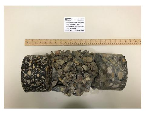
Photo 6: Pavement Core Sample at Test Hole TH19-06
