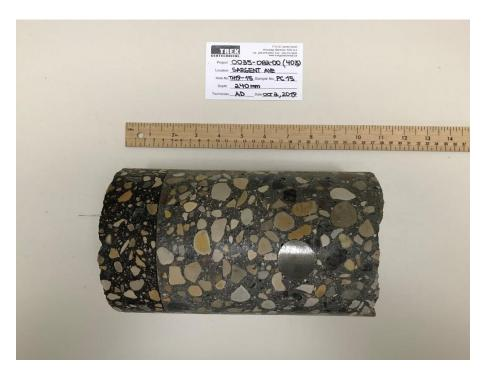
Photo 16: Pavement Core Sample at Test Hole TH19-15
