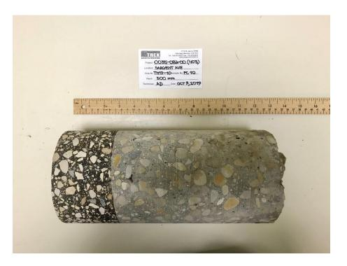
Photo 10: Pavement Core Sample at Test Hole TH19-10
