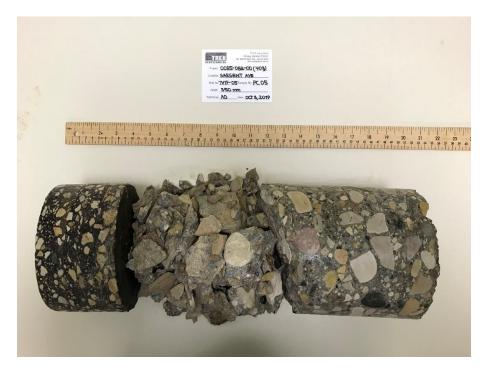
Photo 5: Pavement Core Sample at Test Hole TH19-05
