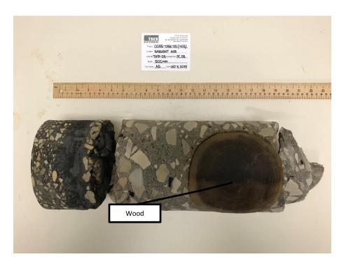
Photo 8: Pavement Core Sample at Test Hole TH19-08
