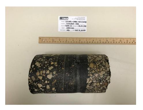
Photo 12: Pavement Core Sample at Test Hole TH19-11B
