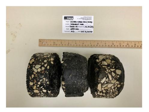
Photo 11: Pavement Core Sample at Test Hole TH19-11A
