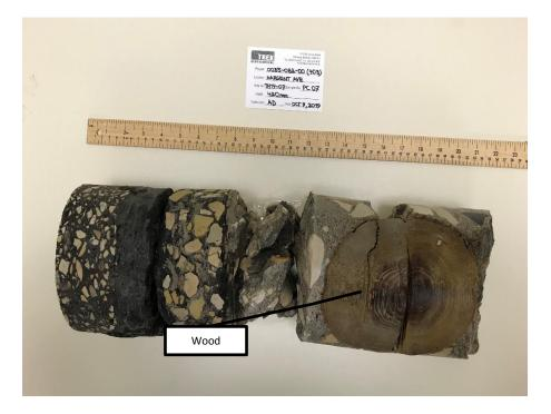
Photo 7: Pavement Core Sample at Test Hole TH19-07
