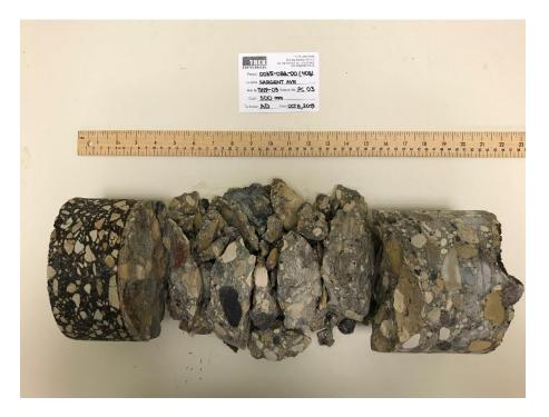
Photo 3: Pavement Core Sample at Test Hole TH19-03
