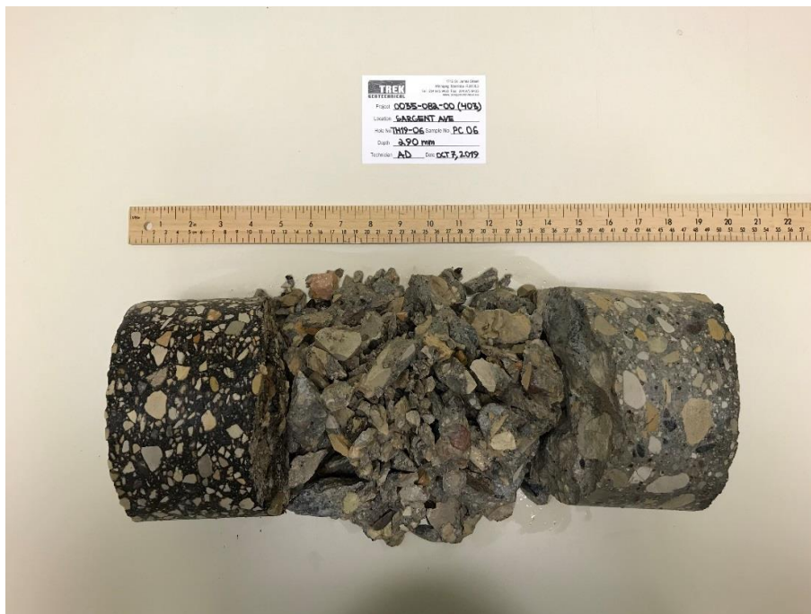
Photo 6: Pavement Core Sample at Test Hole TH19-06
