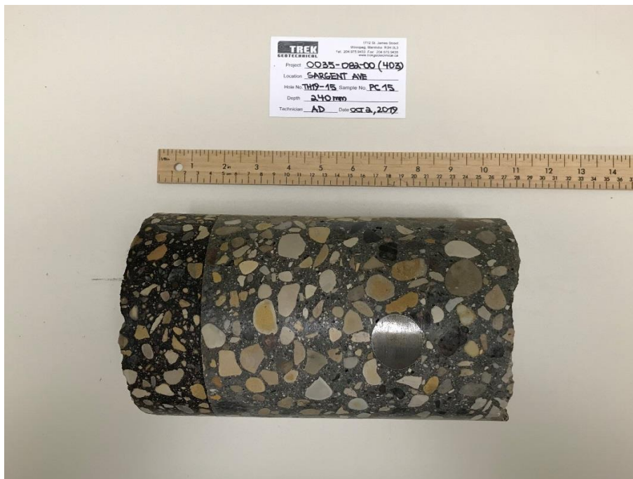
Photo 16: Pavement Core Sample at Test Hole TH19-15
