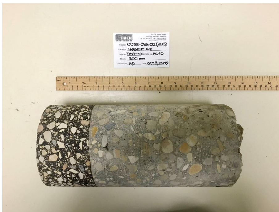
Photo 10: Pavement Core Sample at Test Hole TH19-10
