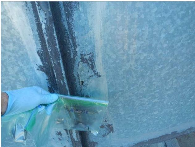
Photo 11. Sample location PS-ACM-03B, black duct mastic, roof of Pumping Station Building.
