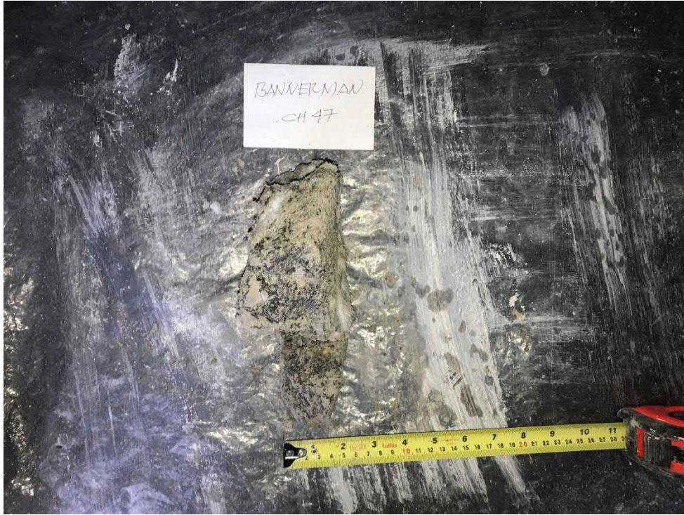
Photograph 45: Core Hole CH20-47 – Bannerman Avenue –Asphalt partially recovered
