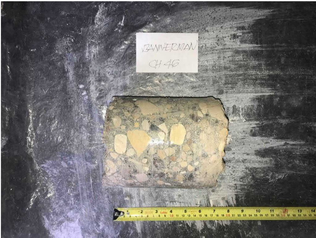
Photograph 44: Core Hole CH20-46 – Bannerman Avenue
