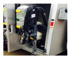
The Equipment Area Cabinets shall be designed to accommodate a back board and stretcher, fire fighter turnout gear, fire extinguisher, various loose fire equipment and must have a sliding SCBA bracket.
