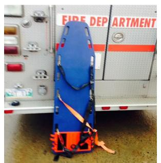
At the floor level, starting at the rear doors and ending between the two (2) wheel wells is the Back Board and Collapsible Stretcher Storage Compartment. This compartment will contain both stretchers side by side
