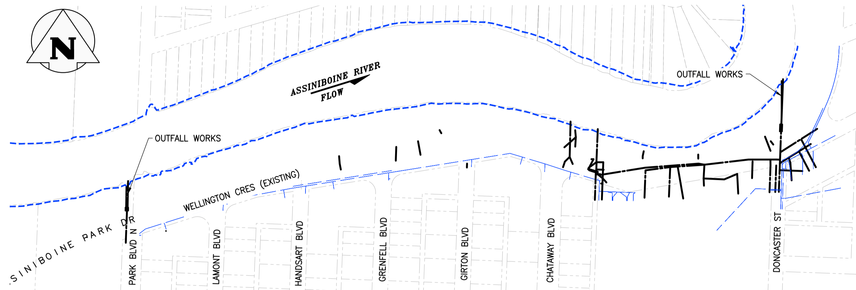
UNDERGROUND (2020 / 2021 WINTER WORKS) (OUTFALLS, SEWER AND WATER) (STAGING DETAILS SEE DWG GE-06)
