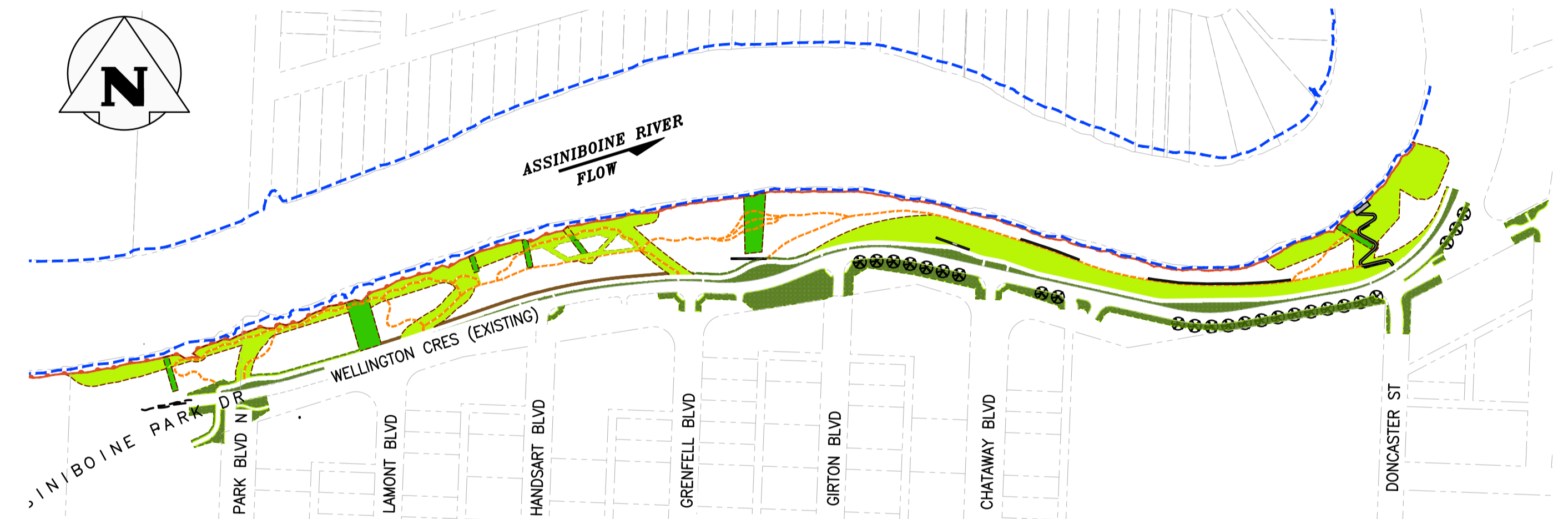
LANDSCAPE (2021 SUMMER WORKS) (RESTORATION, WILDERNESS TRAILS, TENSION CRACK SEALING, DRAINAGE IMPROVEMENTS AND ENHANCEMENT) (STAGING DETAILS SEE DWG GE-09)
