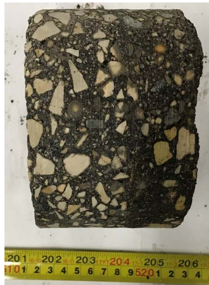
GRO2-04: Intact Core, Profile View
