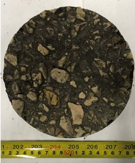
GRO2-05: Intact Core, Plan View
