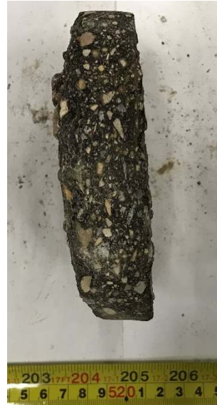
RIL-01: Asphalt Layer, Profile View
