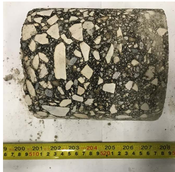
DOW-01: Asphalt Layer, Profile
