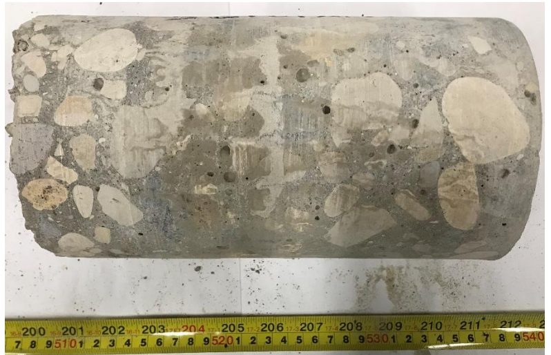
NAT1-02: Intact Core, Profile View
