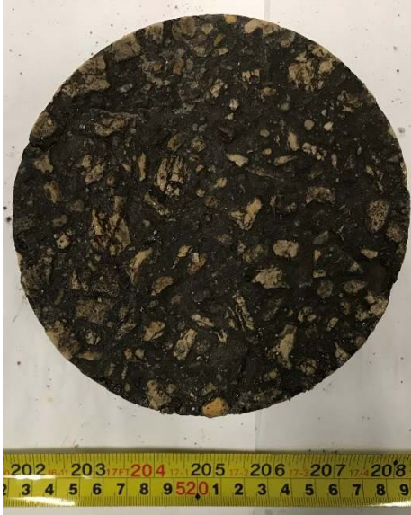
GRO2-09: Intact Core, Plan View
