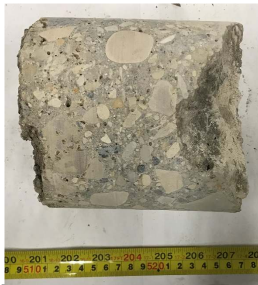
HAR-02: Intact Core, Profile View
