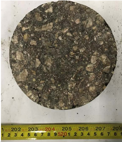
RIL-03: Asphalt Layer, Plan View
