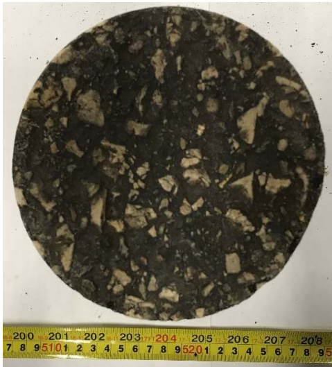
GRO2-02: Intact Core, Plan View
