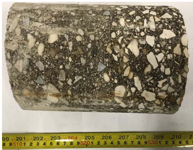
GRO1-03: Asphalt Layer, Profile View
