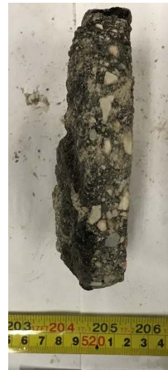
SYR-06: Asphalt Layer, Profile View
