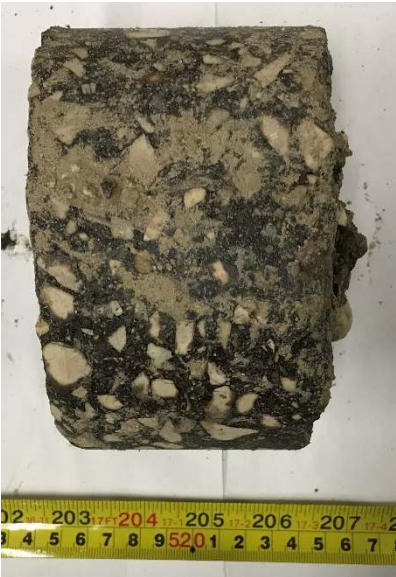
GRO2-01: Intact Core, Profile View
