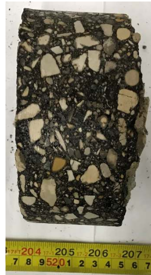
GRO2-07: Intact Core, Profile View
