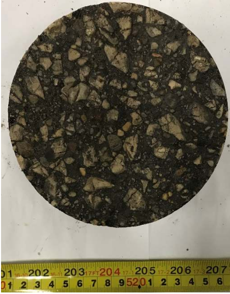
GRO2-03: Intact Core, Plan View
