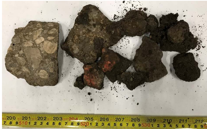
SYR-01: Broken Half Asphalt & Concrete Layer, Plan View
