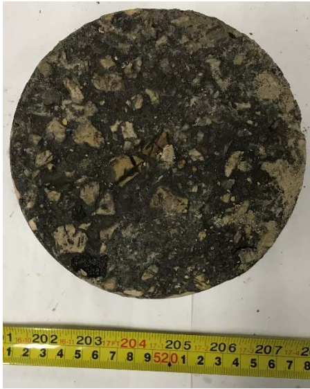
GRO2-01: Intact Core, Plan View
