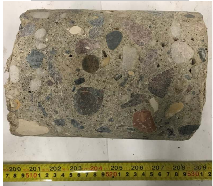
RIL-01: Concrete Layer, Profile View
