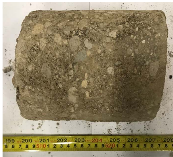
DOW-02: Asphalt Layer, Profile View
