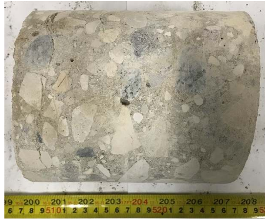
SYR-03: Intact Core. Profile View
