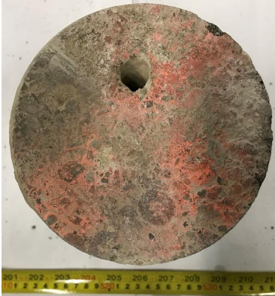
NAT2-01: Intact Core, Plan View
