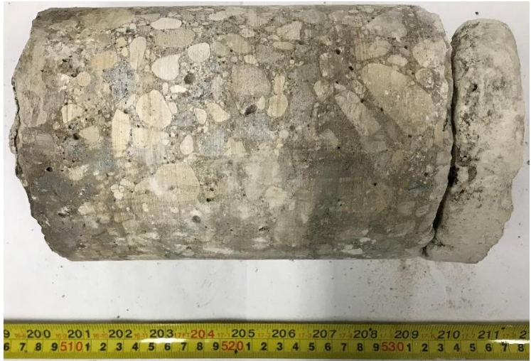
NAT2-03: Intact Core, Profile View
