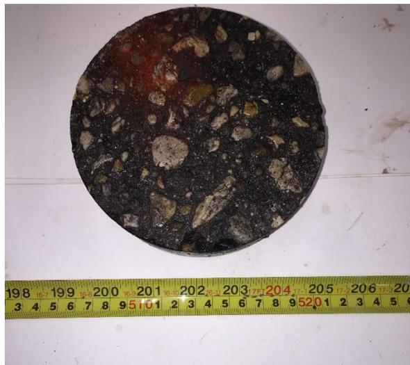
LEO-02: Asphalt Layer, Plan View
