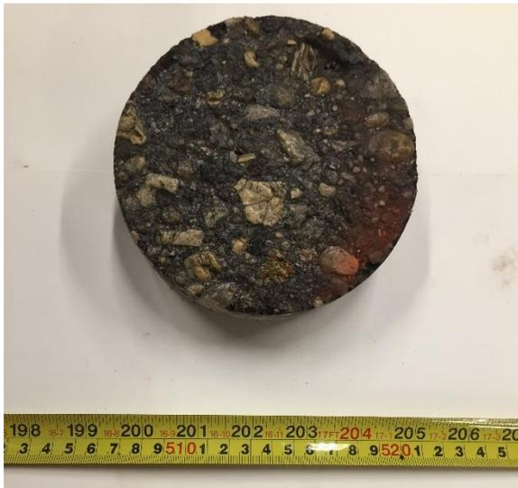
BOW-03: Asphalt Layer, Plan View
