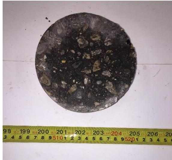
LEO-07: Asphalt Layer, Plan View
