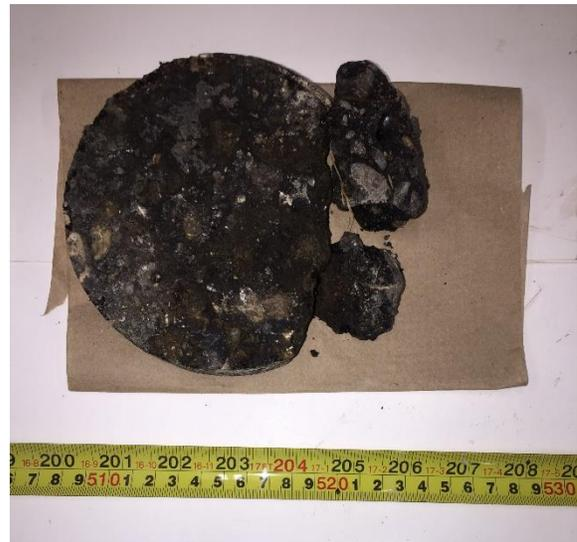
BOW-05: Asphalt Layer, Plan View
