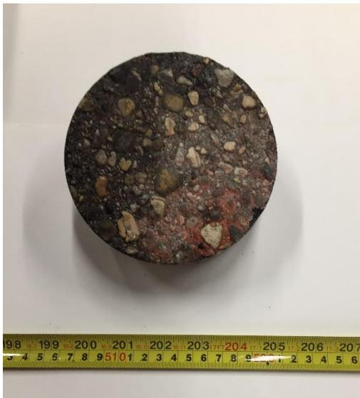
BOW-02: Asphalt Layer, Plan View
