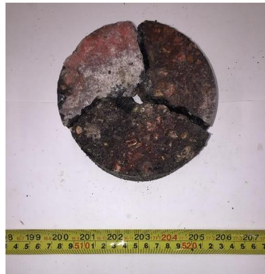
LEO-04: Asphalt Layer, Plan View
