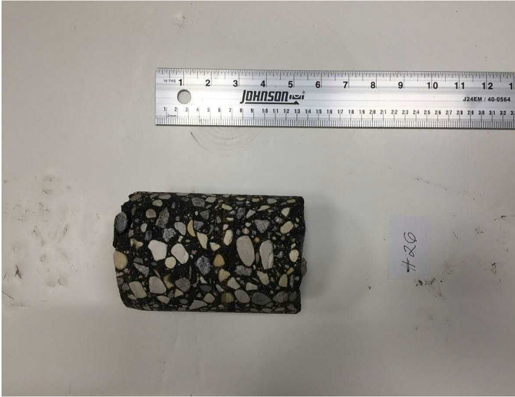
Photograph 13: CH20-26 - Kingston Row (No Concrete Recovery)
