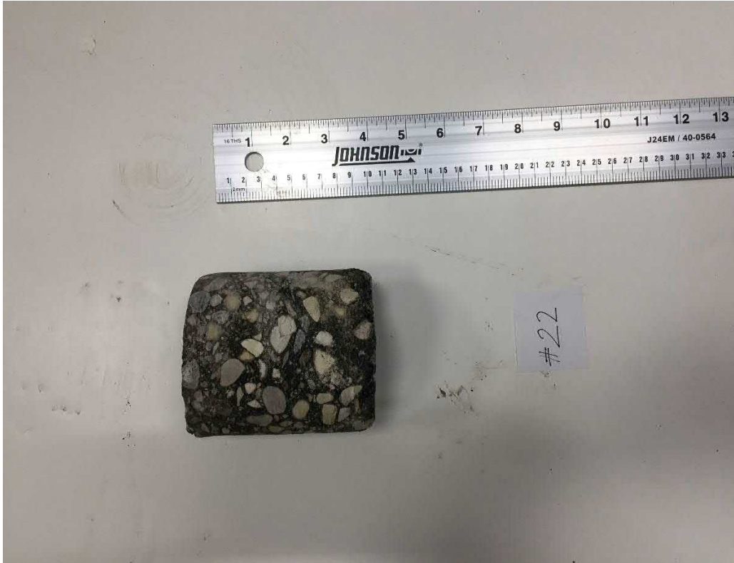
Photograph 9: CH20-22 - Kingston Row (No Concrete Recovery)
